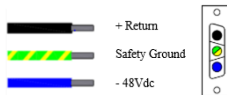
Figure 2-7. DC Input Power Cable Connector
