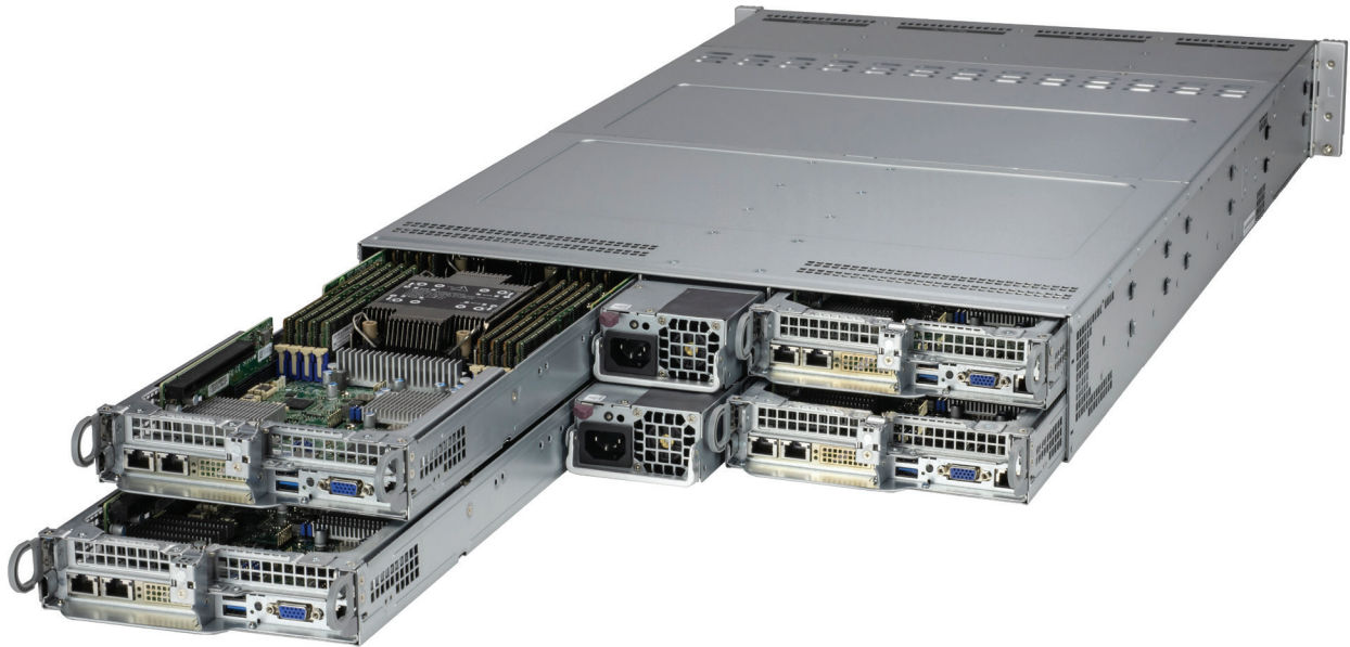
Figure 3-1. Removing the Compute Node
