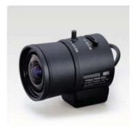
Advanced design engineering and special optic glass adopted, best suited for color, Black and White and Day and Night cameras. Broad range of f2.7-13.5mm, supporting various applications. Wide aperture of F1.3, optimizing the performance at low lighting intensity. High accuracy aspheric lens adopted, achieving the high quality image. Built-in ND filter of T360, supporting high sensitivity cameras.
