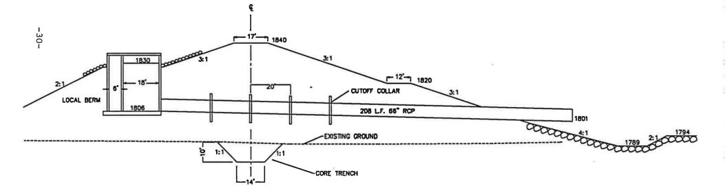
1806 msl. The RCP is 208 feet in length with a 2.5 percent slope with the outlet invert at elevation 1801 msl. The reinforced concrete pipe will consist of thirteen - 16-foot sections. Within the length of the spillway there will be 6 reinforced concrete anti-seep collars. The outlet structure consists of a standard cantilevered outlet with stilling basin.
