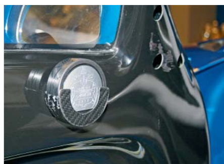
The snus can holder, which is mounted on the inside of the Porsche's driver's door, is designed for a General Onyx can.
