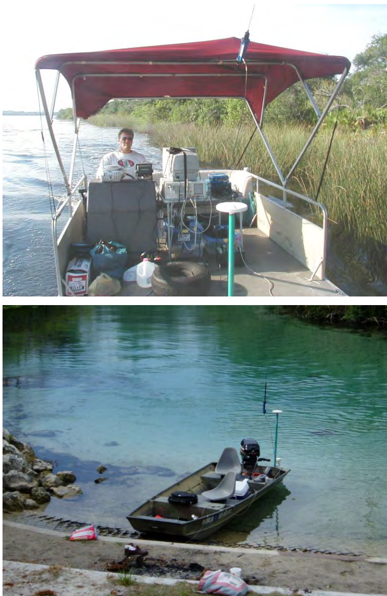
Figure 2. The survey vessels, upper: the pontoon boat; lower: the 15-ft aluminum boat.
