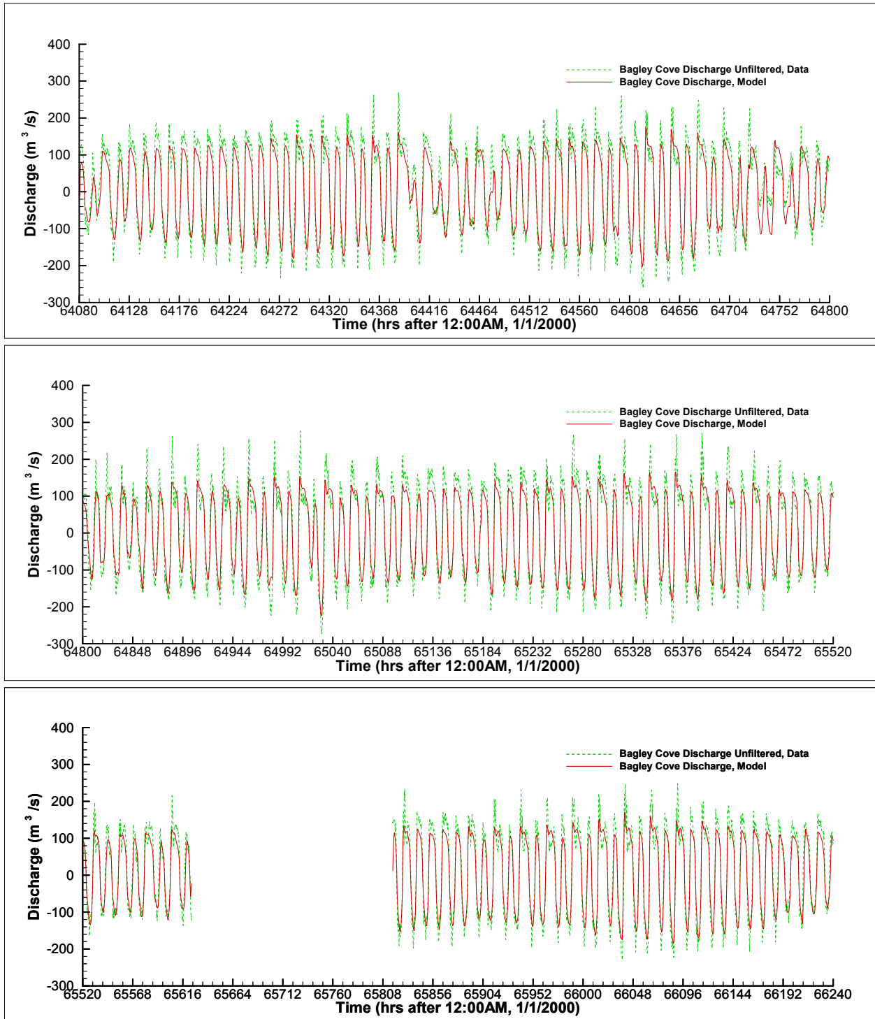
Figure E - 1 Comparison of simulated and measured cross-sectional discharges at Bagley Cove in Crystal River during Hours 64080 – 66240.
