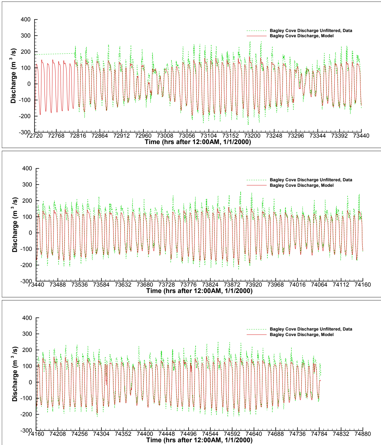
Figure E - 5 Comparison of simulated and measured cross-sectional discharges at Bagley Cove in Crystal River during Hours 70560 - 74880.
