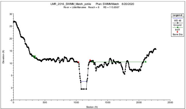
Figure 6-3. Example cross section (Cross Section 115.66 in Reach 8) in the Upper Little Manatee River where the inflection point was associated with a relatively deep channel water depth (i.e., 3.1 ft).
