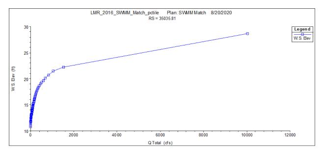
Figure 5-6. Example rating curve for the Upper Little Manatee River at Cross Section 35035.81 (W.S. Elev = water surface elevation, Q Total = flow rate or discharge).
