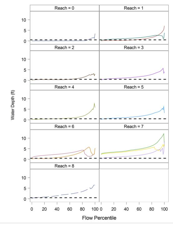
Figure 6-14. Water depth as a function of flow profile under the Baseline condition for 9 reaches in the Upper Little Manatee River. Horizontal reference line indicates a water depth of 0.15 m (0.5 feet). Multiple colored lines indicate station within Reaches 3, 6, and 7 (from Jacobs and JEI 2021d).
