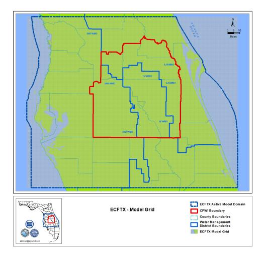
Figure 2-28. Model grid for the East Central Florida Transient Expanded (ECFTX) model domain.
