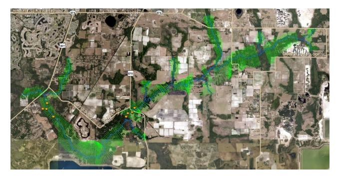
Figure 5-9. The location of 7 sites (yellow circles) where substrate/cover was characterized for the SEFA analyses at a total of 21 cross sections, and all HEC-RAS cross sections (green lines) along the Upper Little Manatee River.
