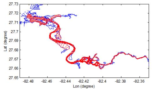
Figure 5-11. The orthogonal grid system (horizontal view) used by the EFDC model for the Lower Little Manatee River estuary.
