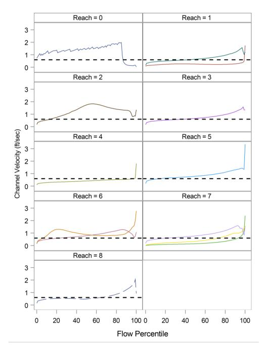
Figure 6-13. Cross-sectional average velocity as a function of flow profile under the Baseline condition for 9 reaches in the Upper Little Manatee River. Horizontal reference line for each reach indicates the critical velocity of 0.6 ft/sec. Multiple colored lines indicate stations within Reaches 1, 6, and 7 (from Jacobs and JEI 2021c).
