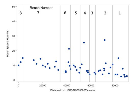
Figure 6-4. Reach specific critical flow values associated with a 0.6-ft (0.18-m) hydrologic depth for fish passage in the Upper Little Manatee River (from JEI 2018a).
