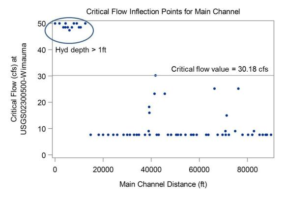
Figure 6-2. Critical flow for each HEC-RAS cross section (y axis) as a function of distance from the downstream USGS Little Manatee River at US 301 near Wimauma, FL (No. 02300500) gage (from JEI 2018a).
