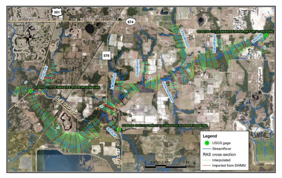
Figure 5-5. Seventeen river reaches (0 to 8 are the reaches for the main stem) and 478 cross sections in the 2018 Upper Little Manatee River HEC-RAS model. Locations of available US Geological Survey gages associated with the Upper Little Manatee River are shown.
