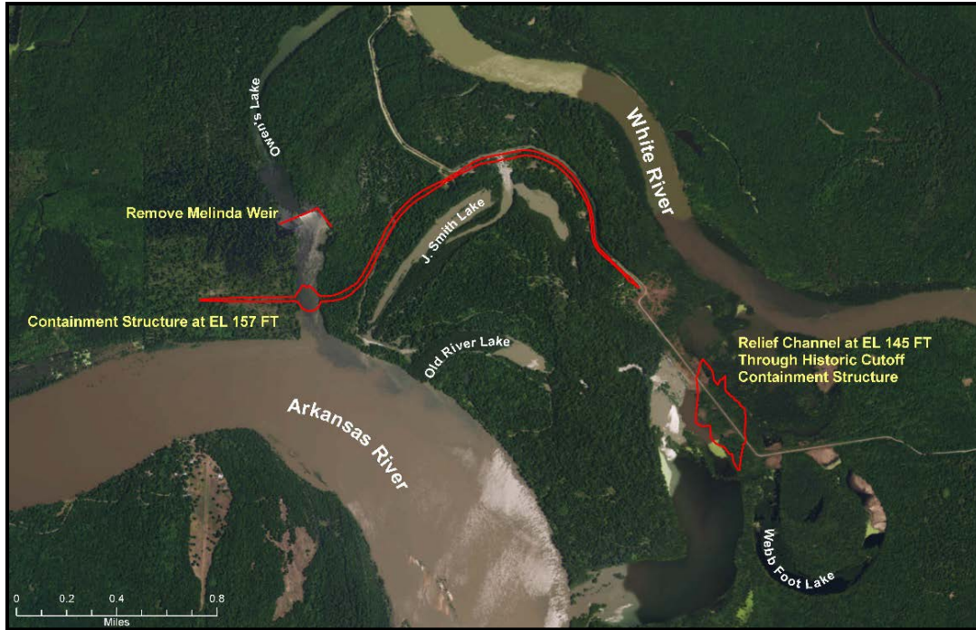
1 Figure B: Alternative 1 Structure Alignment
