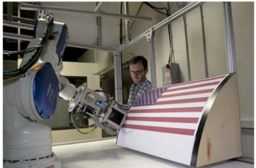
Figure 1: Inkjet EoAT on laboratory robot
