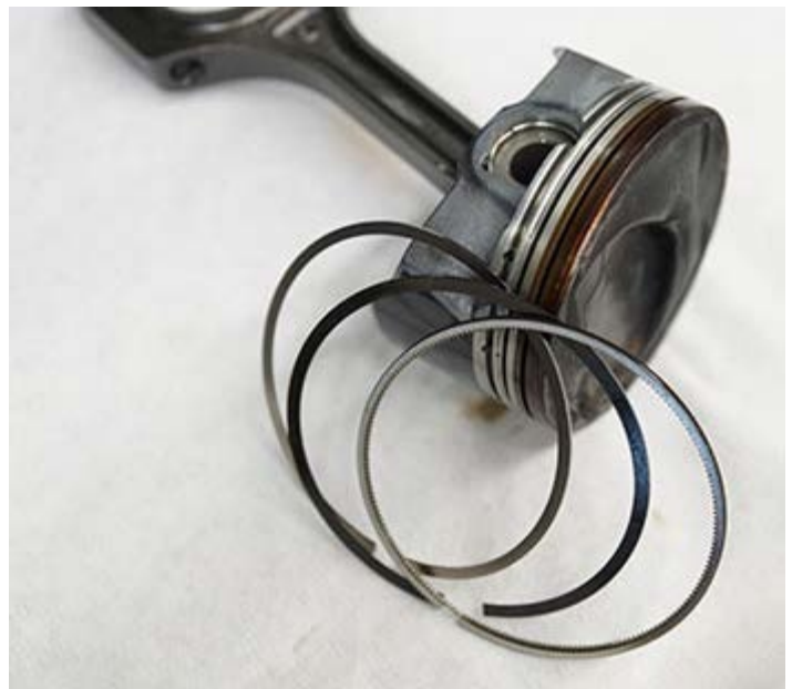
Figure 1: Engine piston rings after removal from engine
