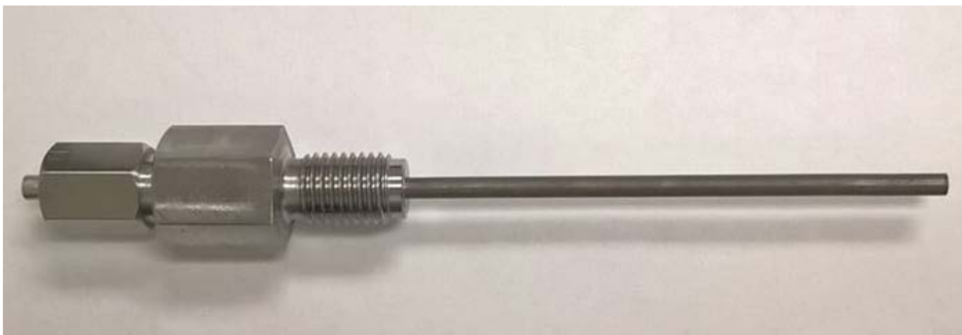
Figure 2: Dual-fuel, ionization current probe.
