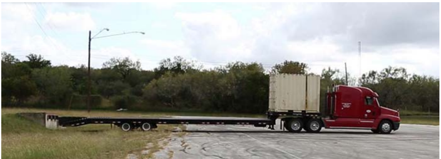
Figure 1: SwRI Class VIII truck autonomously backed up to a loading dock.
