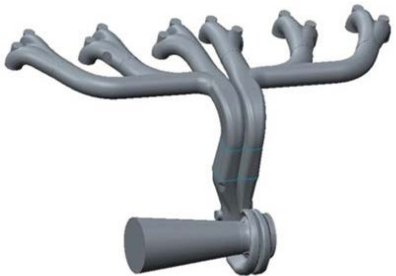
Figure 1: Three-dimensional computational fluids model of turbocharger system.
