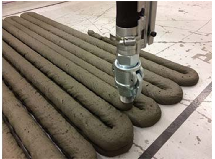
Figure 1: Example of 25mm wide x 17mm thick layer-by-layer serpentine pattern testing.
