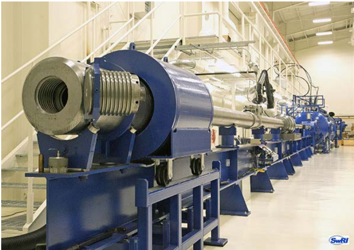
Figure 1: The centerpiece of a new 7,050 square foot facility at SwRI is a two-stage light-gas launcher featuring a 38-mm-diameter launch tube (1.50 caliber) with the ability to achieve velocities up to 7 kilometers per second (15,660 miles per hour).
