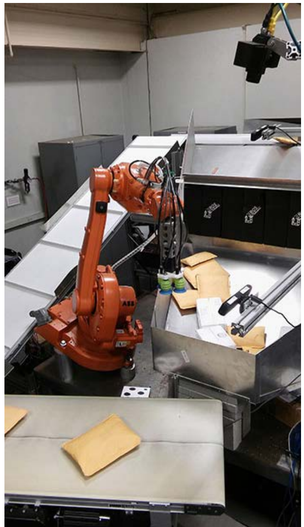
Figure 1: Parcel sorting work cell with ABB robot, vacuum gripper, and 2-D/3-D sensors.
