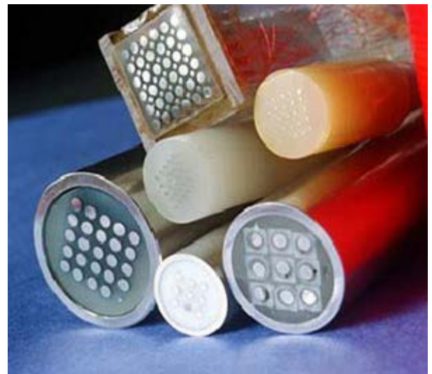
Figure 2: Examples of multi-electrode corrosion probes
