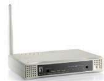
WBR-6603 150Mbps Wireless ADSL2+ Modem Router
