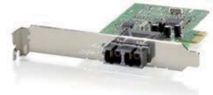
FNC-0115 100BASE-FX MMF Optic PCI Express Card (SC)
