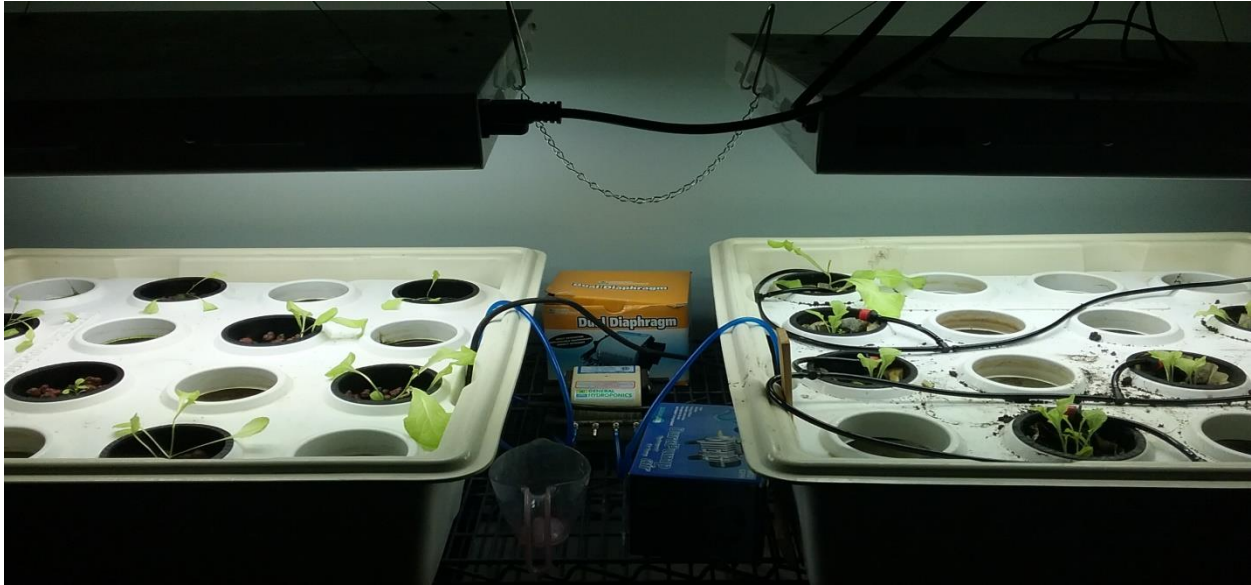
Figure 1: Design of both Growing Treatments. The Deep Water Culture (DWC) treatment is shown to the left , and the Soil Treatment is shown on the right .
