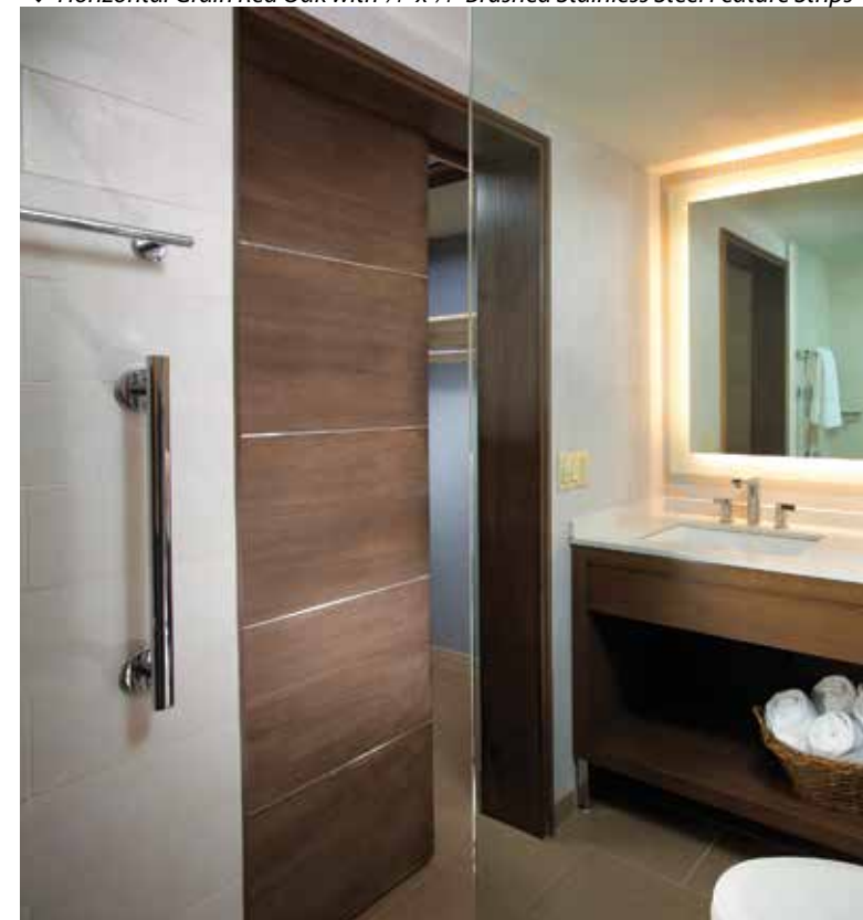
▼ Horizontal Grain Red Oak with 1/4" x 1/4" Brushed Stainless Steel Feature Strips
