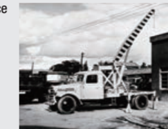
The first hydraulic truck crane, the OC-2
