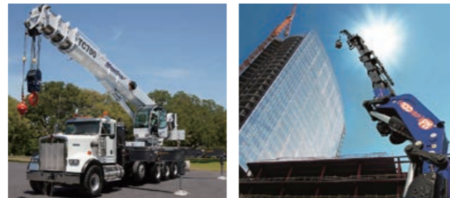
Boom truck crane
