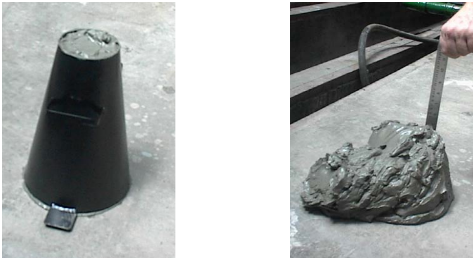
Figure 17: Slump cone test of GyöngyöSOROSZI flotation tailings at solid concentration of 50% (V/V).
