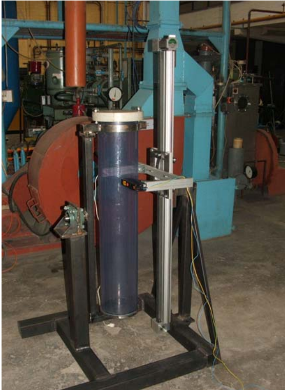
Figure 39: The pilot-scale settling column with vibration.
