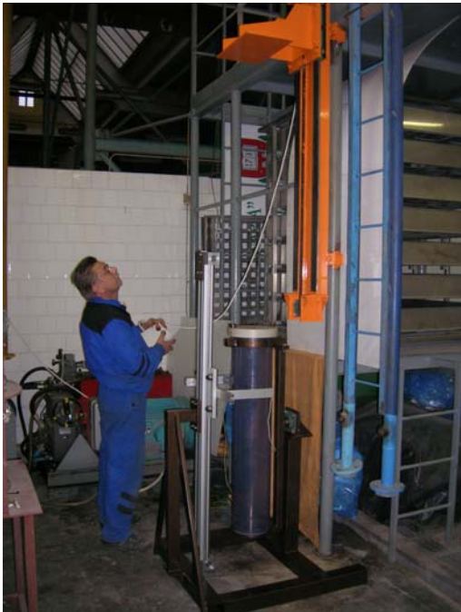
Figure 41: The linear motor's traversing system
