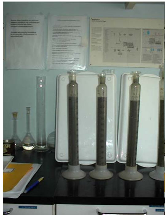
Figure 15: Column settling tests of Gyöngyösoroszi tailings material (without flocculating reagent).
