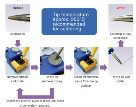
NOTE: When the tip temperature is over 400°C, even if the oxidation film is removed by "HAKKO FT-700 tip polisher", the tip can turn to be oxidized quickly again.
