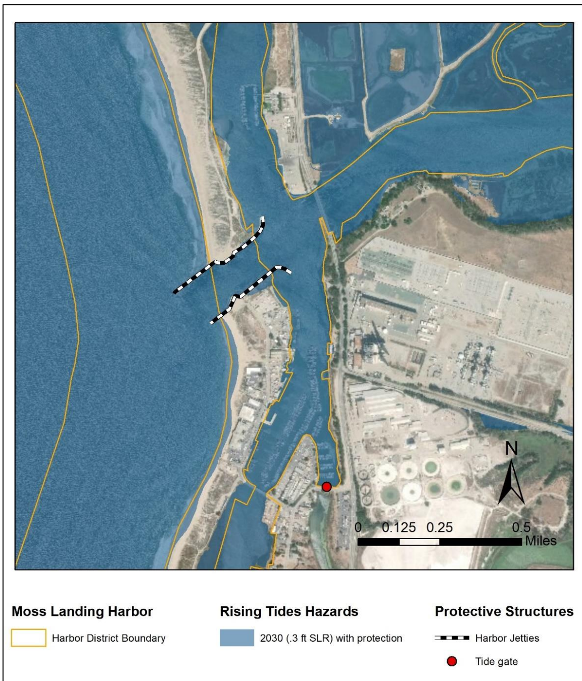
Figure 5. Flooding associated with 2030 increases in sea level (0.3ft)
