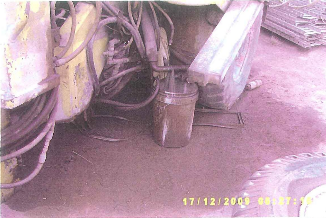
Photo 15: Hydraulic Oil Leaking from disused Equipment in the Coyote Plant Laydown area.
