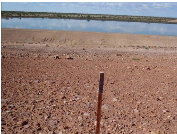
Plate 5: Coyote WRL, west end of northern slopes, trial control surface, no topsoil, approximately four years after establishment (TGNL 2012c)
