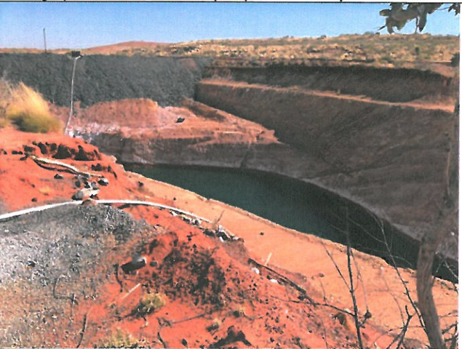
Photograph 17 – Pit 1, dewater from Pit 2 pumped in
