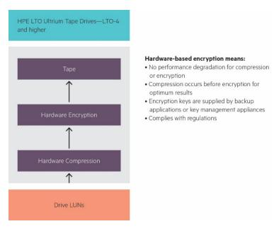
Figure 6. Hardware-based data encryption
