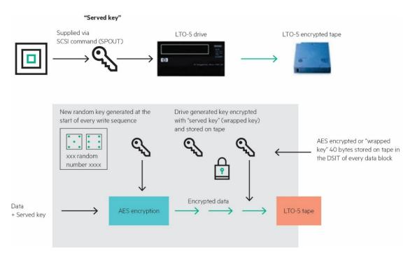
Figure 7. LTO-5 Ultrium Tape Drive-wrapped key
