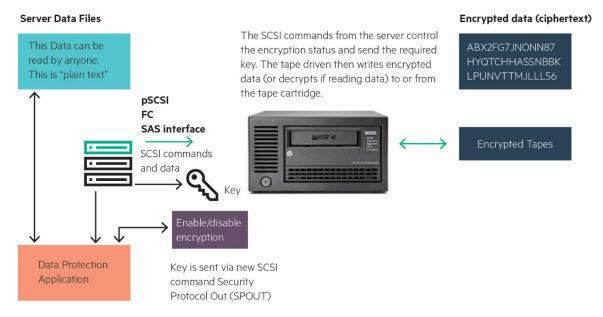
Figure 1. Overview of the HPE StoreEver LTO Ultrium Tape Drive Encryption process
