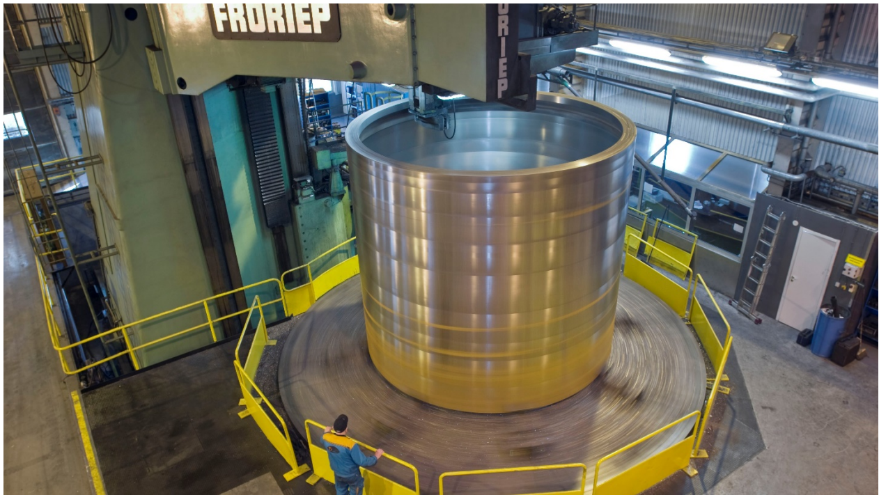
Figure 4. Machining of yankee shell.
