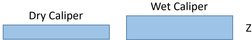
$$V_{\text{swelling}} = V_{\text{sheet wet}} - V_{\text{sheet dry}}$$
