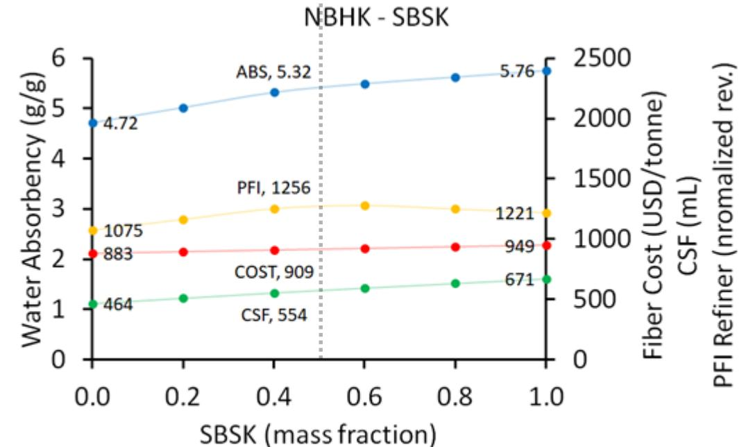
● Absorbency (g/g) ● Fiber Cost (USD/tonne) ● CSF (mL) ● PFI Refiner (rev.)
