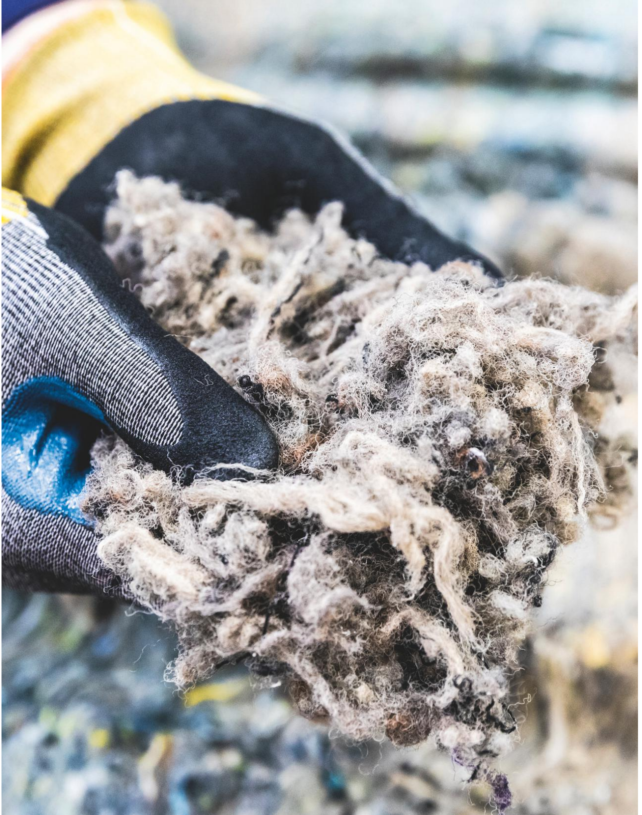
Fluff - high purity yarn (95%) - is generated by Tarkett's carpet recycling center at Waalwijk, The Netherlands.
