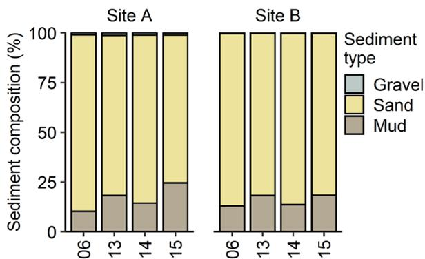
Fig. 4. Sediment particle grain size analysis showing percentage composition of mud (<63µm), sand (<2mm to ≥63µm) and gravel (≥2mm).
