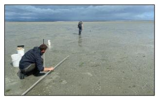
Example of measuring sediment plate depth. A straight edge is used to account for small scale irregularities in the sediment surface. Depth is measured to the nearest millimeter (at least in triplicate) and recorded as an average per plate.
