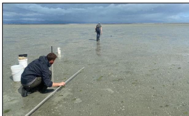
Example of measuring sediment plate depth. A straight edge is used to account for small scale irregularities in the sediment surface. Depth is measured to the nearest millimeter (at least in triplicate) and recorded as an average per plate.
