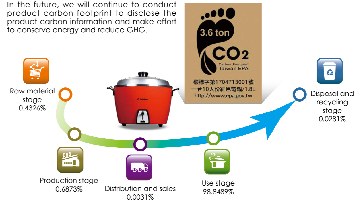
▲ Carbon information on each life cycle stage for multi-function cooker (TAC-10L-SR)
