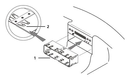
Fig. 5 - 12: Assembling installation frame in the radio compartment
