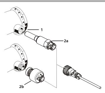
Fig. 5 - 9: Installing the KITAS 2171 motion sensor
