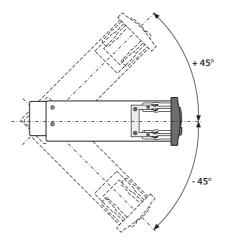
Fig. 5 - 2: Installation angle of the DTCO 1381
