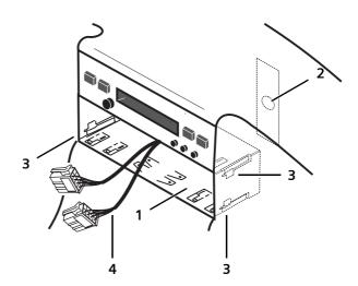
Fig. 5 - 13: Checking the radio compartment with the installation frame
