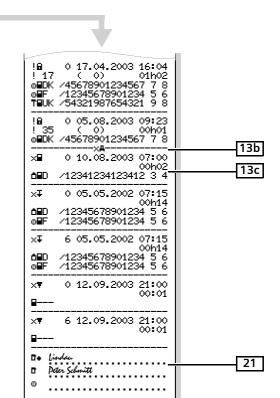
Fig. 14 - 6: Printout example: DTCO 1381 events / faults
