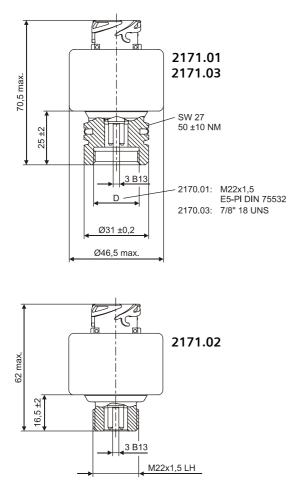
Fig. 2 - 12: Installation dimensions 2171.0x Standard version
