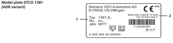
Fig. 6 - 3: Model plate DTCO 1381 (ADR variant)
