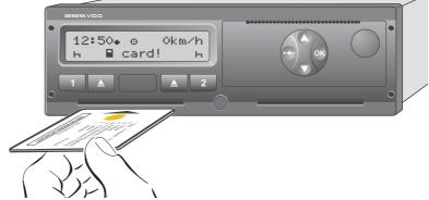
Fig. 10 - 2: Inserting workshop card
