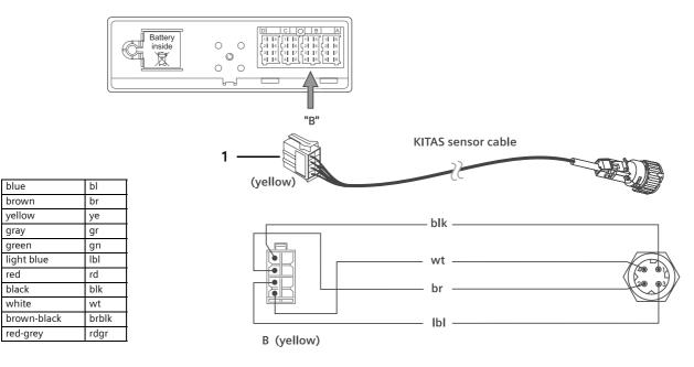
Fig. 6 - 6: KITAS 2171 intrinsically safe circuitry
