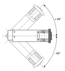
Fig. 2 - 2: Permissible installation angle of DTCO 1381
