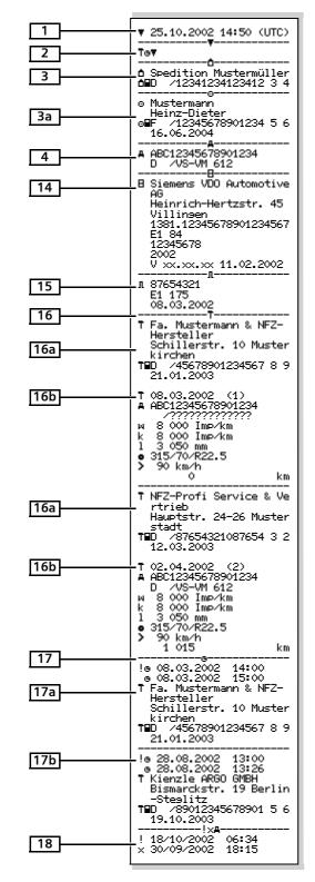
Fig. 14 - 8: Printout example: Technical data of the DTCO 1381
