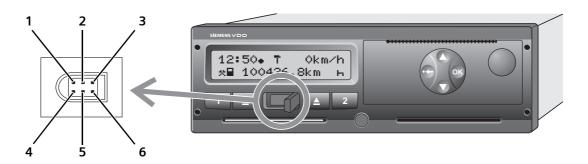
Fig. 2 - 5: DTCO 1381 pin assignment of calibration and download interface
