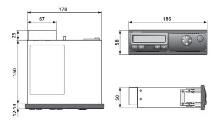
Fig. 2 - 1: Installation dimensions of DTCO 1381
