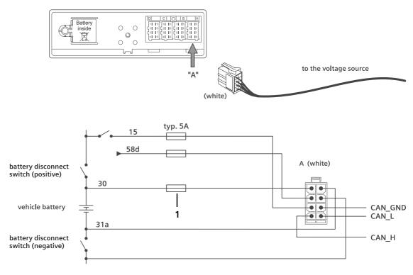
Fig. 6 - 5: Power supply attachment diagram DTCO 1381 (ADR variant)
