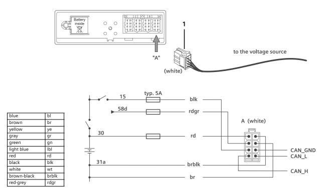
Fig. 5 - 17: Connect the DTCO 1381 connection plug A
