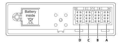
Fig. 2 - 4: Pin assignment DTCO 1381
