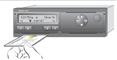
Fig. 3 - 1: Inserting workshop card
