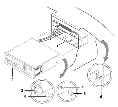
Fig. 5 - 18: Mounting the DTCO 1381 in the radio compartment
