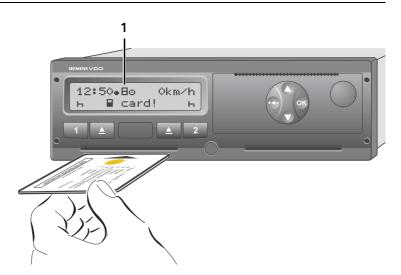
Fig. 9 - 1: Inserting workshop card
