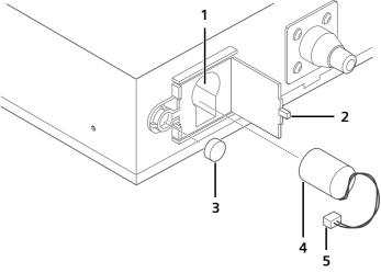
*Fig.* 12 - 2: *Replacing the buffer battery*
