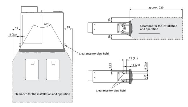
Fig. 5 - 3: Clearance for the installation and operation of the DTCO 1381
