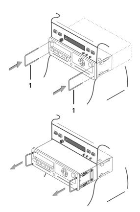
Fig. 12 - 1: Removing the DTCO 1381 from the radio compartment
