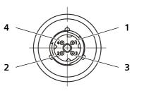
Fig. 2 - 13: Pin assignment KITAS 2171.0x Standard version
