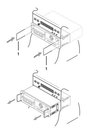
Fig. 5 - 19: Removing the DTCO 1381 from the radio compartment
