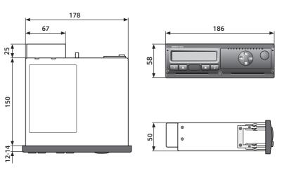
Fig. 5 - 1: Installation dimensions of DTCO 1381
