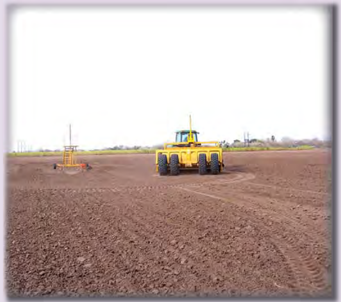
Global positioning land leveling system
