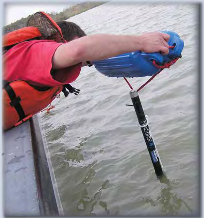
Deploying 24-hour DO monitors
