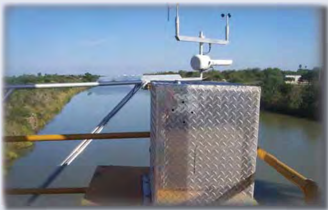
Automated continuous water quality monitoring station on the Arroyo Colorado Tidal at Rio Hondo
