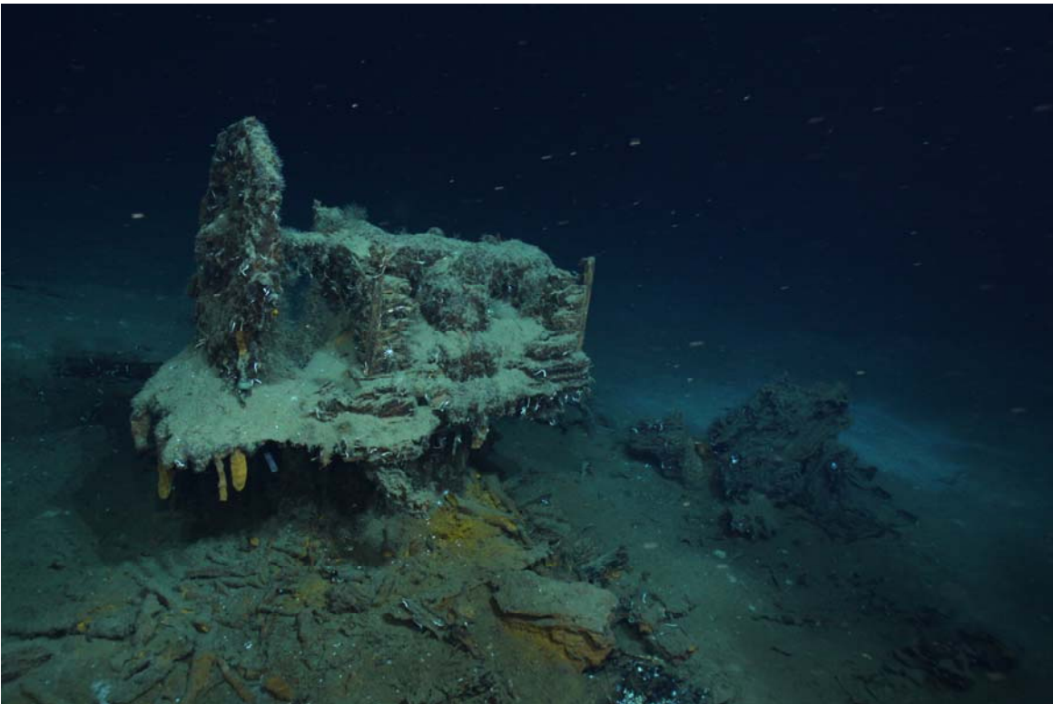
Figure 7-78. Image of the intact steering mechanism on the 7,000 Foot Wreck.
