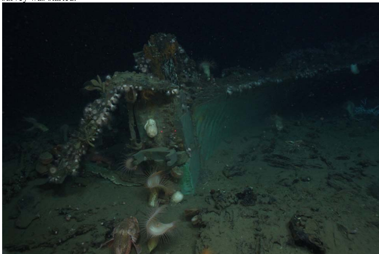
Figure 7-83. View of the sternpost showing the pintle and gudgeon remnants.
