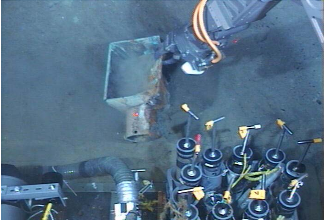
Figure 7-94. Jason II recovering one of the ship's navigation lanterns from the Green Lantern Wreck. .
