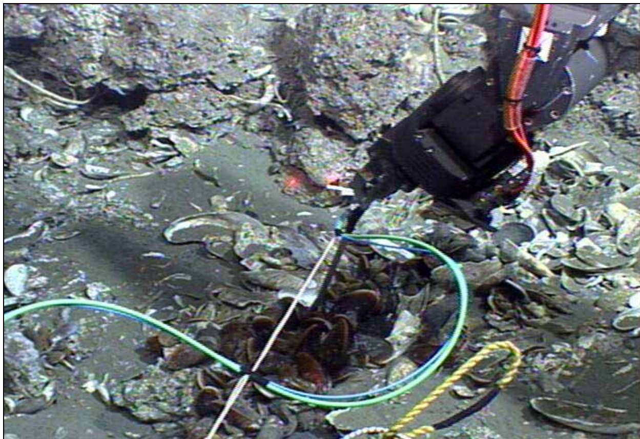
Figure 7-45. Mass Spec readings over mussel bed
