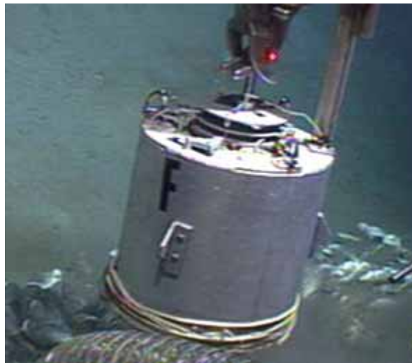
Figure 3-8. Mussel pot deployed with manipulator arm of JASON .
