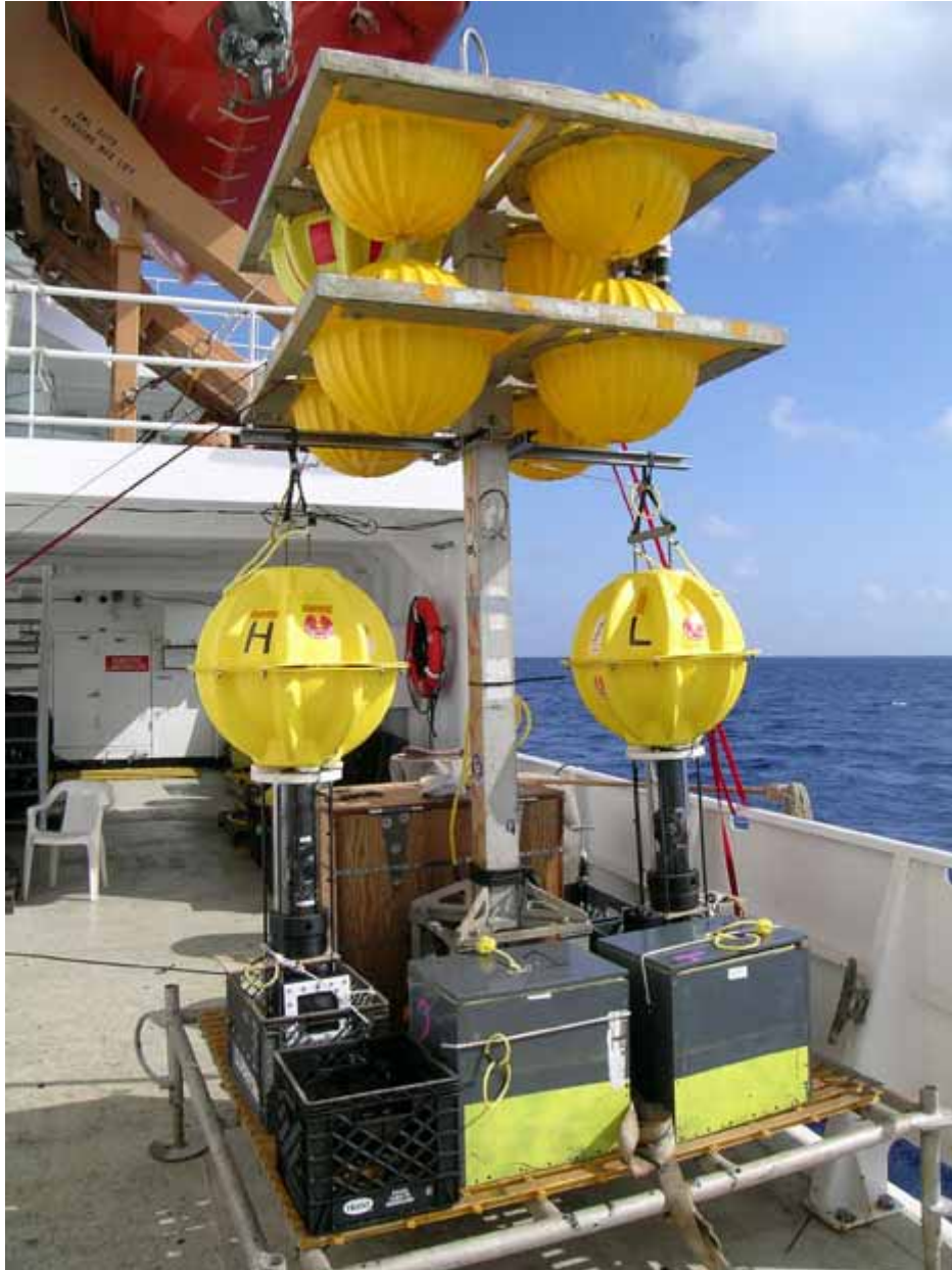
Figure 3-10. Two time-lapse cameras are loaded on the elevator and ready for their initial deployment.
