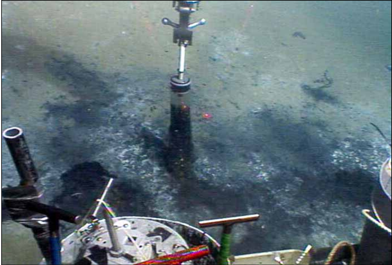
Figure 7-12. Collecting push-core samples in bacterial mat
