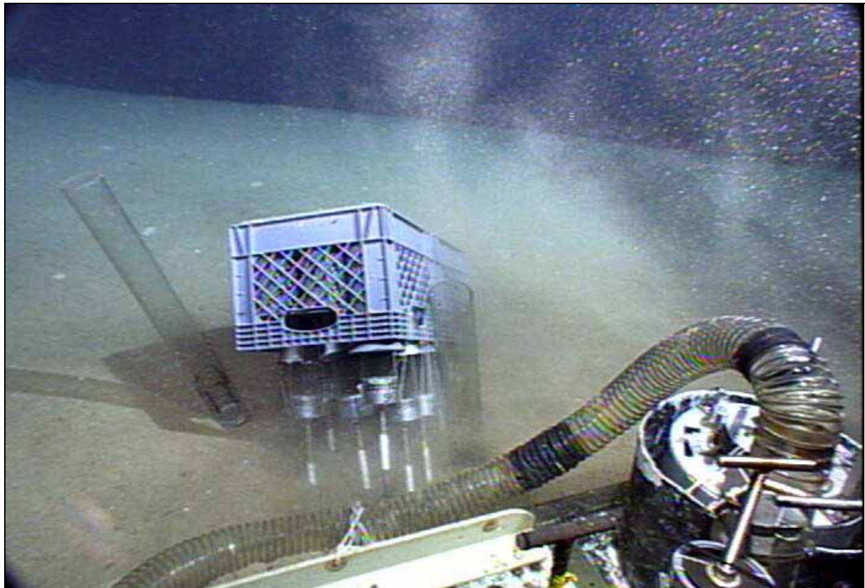
Figure 7-30. Core rack falls off Jason
