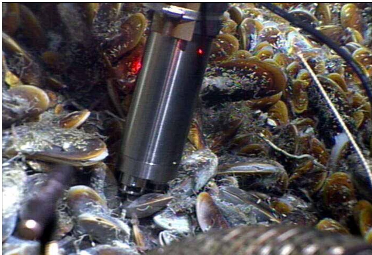
Figure 7-40. Methane Sensor deployed in mussel bed
