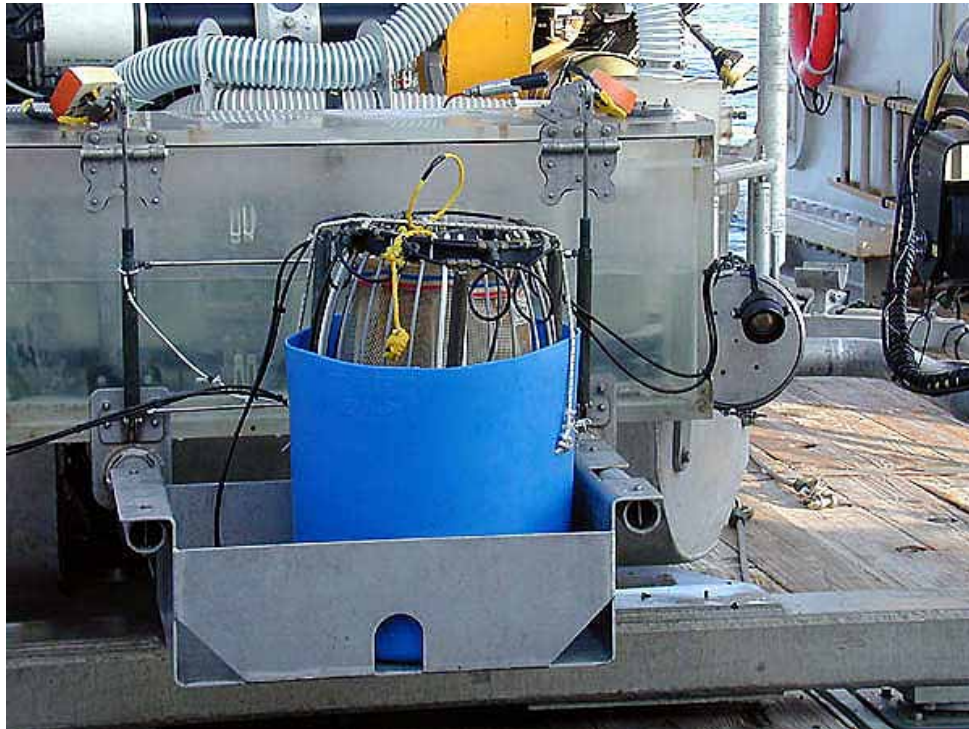
Figure 3-5. The "Bushmaster", a collecting net designed to recover an entire bush of tube worms including all the species that live in association with the worms.
