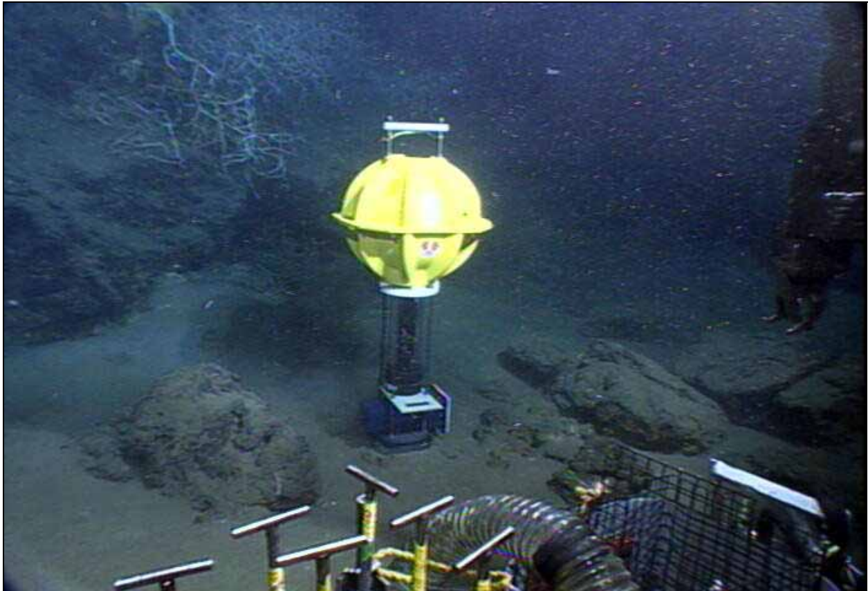
Figure 7-43. Rotary camera deployed for 2 months at coral bed
