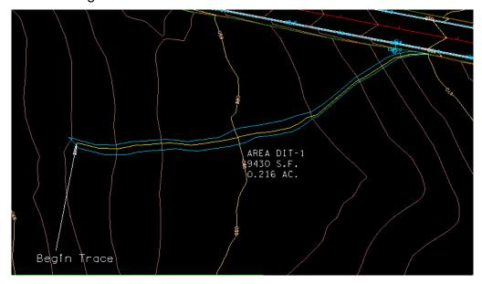
**NOTE:** The drainage area should be broken into sections for long ditches, however, for short ditches; determine the area from the most downstream point (i.e. the stream outlet).
