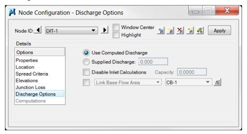
**NOTE:** For short ditches where only a single drainage area is utilized, the **Link Base Flow Area** option should be toggled ON and set to add the discharge for that area. It is then toggled off at the ditch outlet. If this is not toggled OFF at other nodes beyond the beginning, the discharge will accumulate at each node and not accurately represent the area's discharge.
