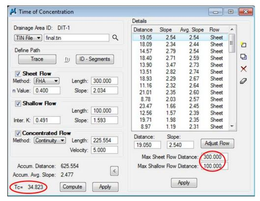
Make settings as shown for Max Sheet Flow and Max Shallow Flow. We will use these settings for all the ditch areas.
