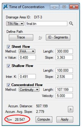
The calculated Time of Concentration is **GREATER** than the minimum of 5 minutes; therefore the Time of Concentration will automatically be filled in after hitting Apply with NO further steps required
