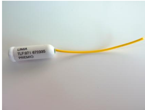
Fig. 5.1.- Data storage tag used on juvenile meagres. The yellow tube remains externally to make the tag visible by the fishermen.
