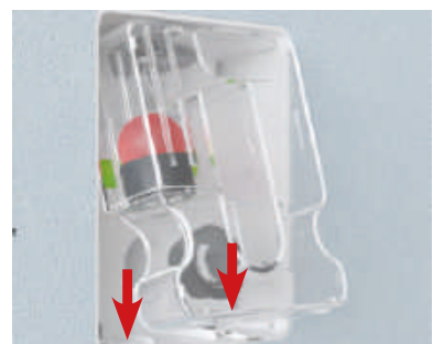
Press the tabs downwards and remove the siphon. Tilt the siphon, insert it into the niche and press it till the tabs go up.
