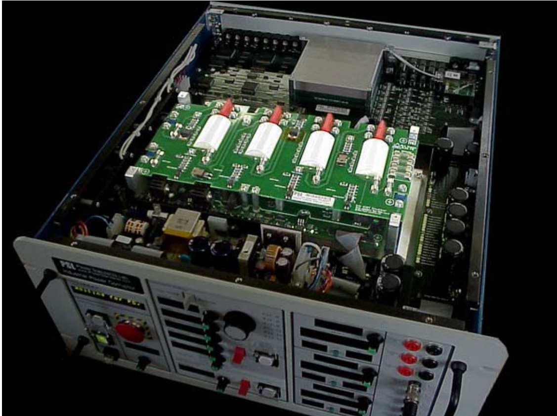
Figure 22: Industrial Power Corruptor (IPC)
