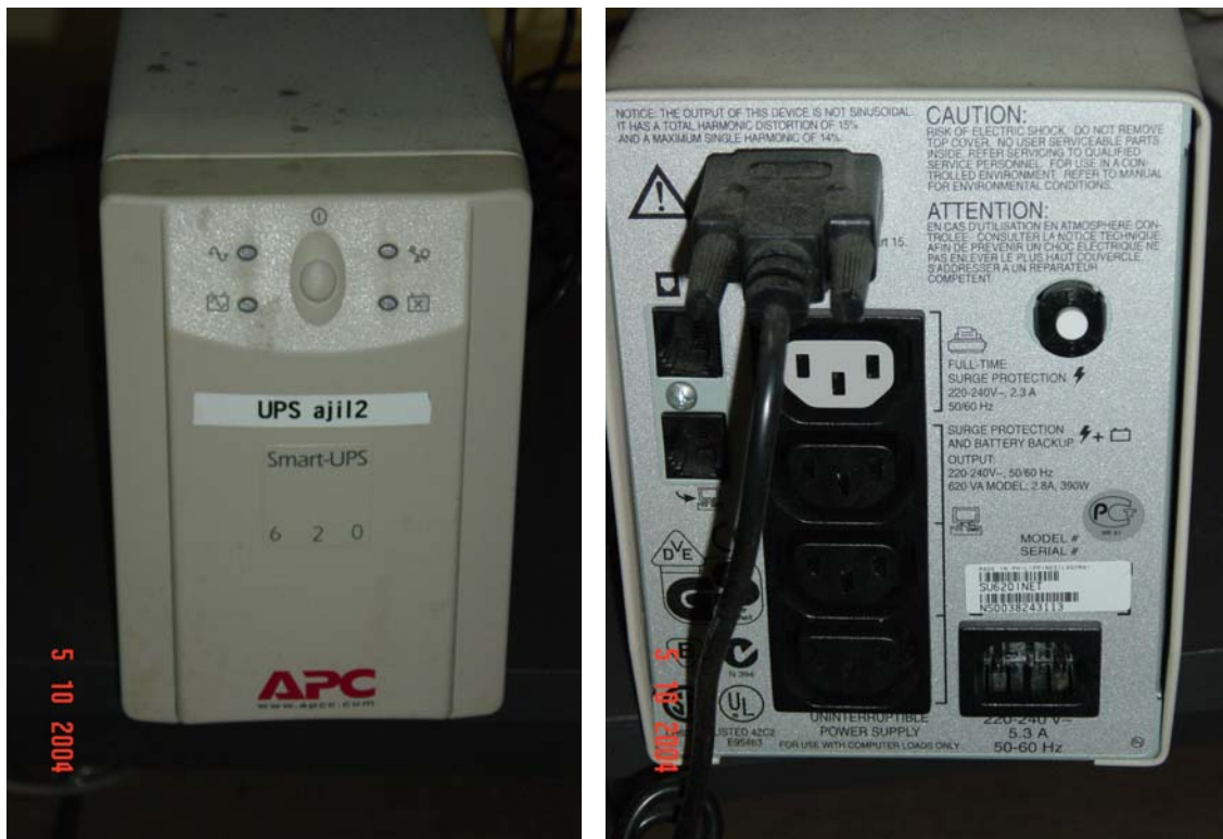
Figure 30: Uninterruptible Power Supply (UPS)
