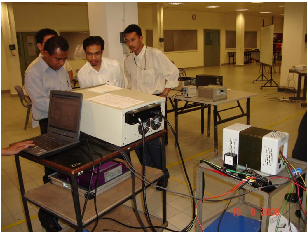
Figure 23: Voltage immunity test
