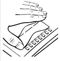
To label the fixed function keys ( $\rightarrow$  page 3), punch out the **small** preprinted labeling card. Insert the card and cover it with the plastic foil supplied (matt side up), as shown in the drawing.
