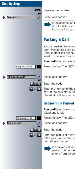
If the connection between the two other parties is not established within 45 seconds, the call from the first part returns to you (recall).
