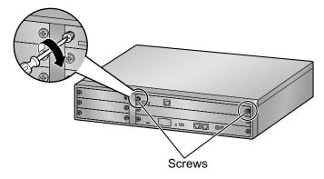
**4.** To remove the card, reverse the procedure above.
