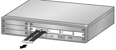
To doorphones/door openers/ external sensors/external relays
