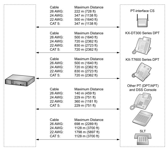
\* The maximum cabling distance from the PBX is the same even when the KX-DT300/KX-T7600 series DPT is the master DPT on the Digital XDP connection.
