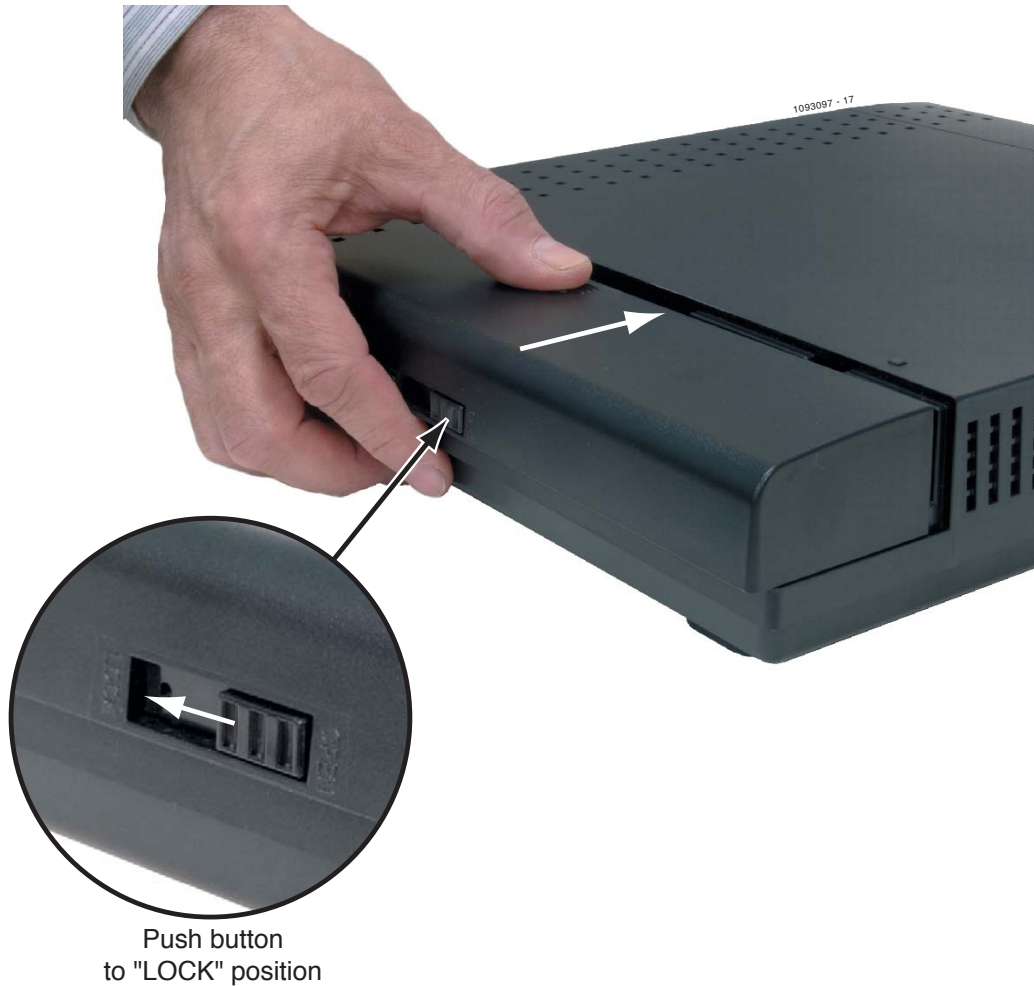
Figure 25: Reinstalling the Cover
