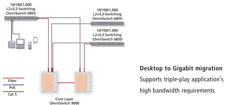
The OmniSwitch 6850s are ideal for use at the edge because of their compact fixed form factor design suitable for closets. Their modular expandability, flexible configuration provides an easy path to scale any workgroup up to 384 10/100/1000 ports and 16 10GigE ports in a single stack to support campus wiring closet requirements.
