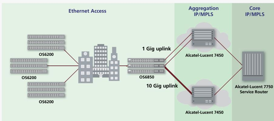
The OmniSwitch 6850s are well suited for residential or metro Ethernet triple-play access networks, which demand user-differentiated, high-speed Internet, voice and video services support. In addition to OmniSwitch 6850 resiliency and high performance, the AOS offers a number of features to provide secure access and traffic control for residential deployments.
