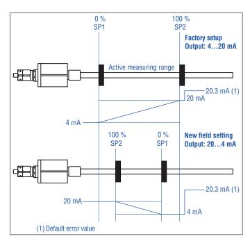
Fig. 38: Start and end position, adjustment  $\slash$  reversal of measuring direction
