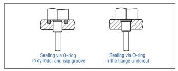
Fig. 7: Possibilities of sealing
