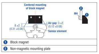
Fig. 14: Mounting of block magnet (part no. 403 448)
