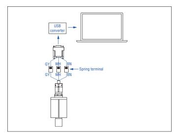
Fig. 32: Connect PC programmer
