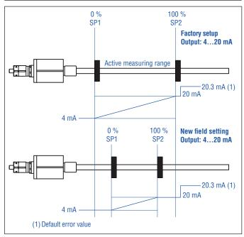
Fig. 37: Adjust start and end position
