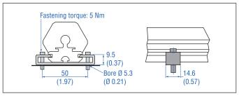
Fig. 10: Mounting clamps (part no. 400 802) with cylinder screw M5×20
