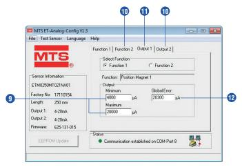
Fig. 35: Example of tab controls
