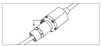
Fig. 20: Grounding via ground lug (version E)
