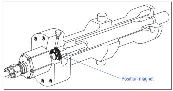
Fig. 6: Sensor in cylinder
