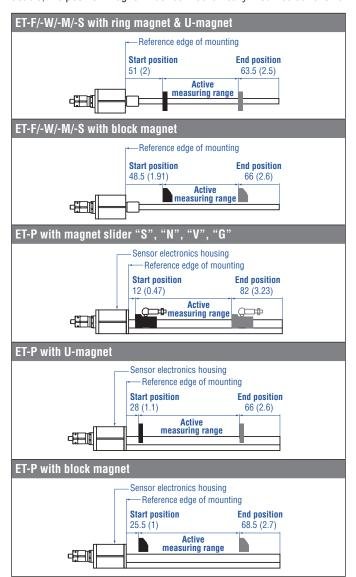
Fig. 17: Start and end positions of magnets
