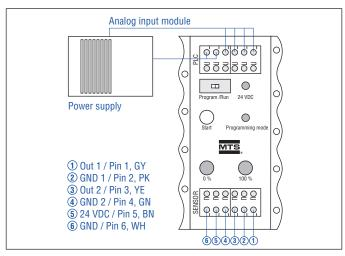
Fig. 29: Connect cabinet programmer (see connector wiring Fig. 21)
