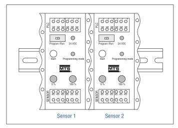
Fig. 28: Dimensions:  $10 \times 55 \times 31$  mm ( $0.39 \times 2.17 \times 1.22$  in.); material: Aluminum, side caps PA 6.6 FR; connection type: Spring terminals, max. 1,5 mm²; ingress protection: IP20
