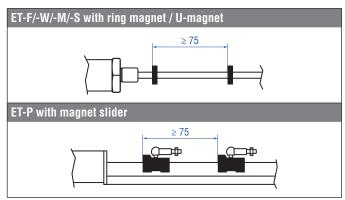
Fig. 18: Examples: Minimum distance for multi-position measurement
