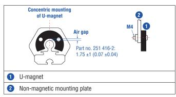
Fig. 13: Mounting of U-magnet (part no. 251 416-2 or part no. 201 553)
