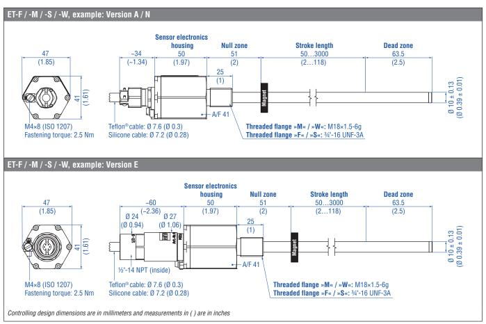
Fig. 4: Temposonics® ET (rod sensor) with ring magnet
