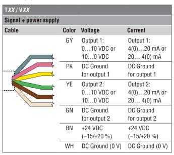
Fig. 21: Connector wiring TXX / VXX
