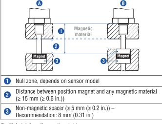
Fig. 15: Installation with magnetic material
