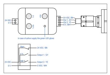
Fig. 24: Connect hand programmer (see connection wiring Fig. 21)
