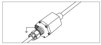
Fig. 19: Grounding via ground lug (version A, N)
