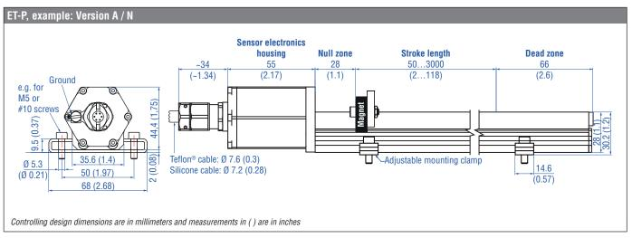
Fig. 9: Temposonics® ET (profile sensor) with U-magnet
