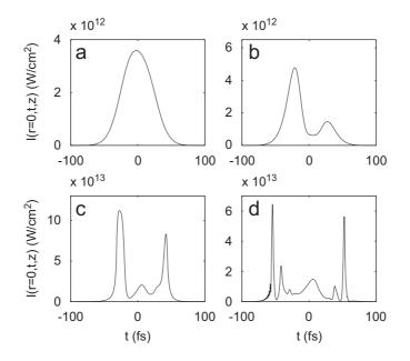
Fig. 24. Pulse temporal profile at successive propagation distances during filamentation. (a) The initial pulse. (b) The pulse splits into two when it propagates beyond the nonlinear focus. (c) The substructures are shortened and stiffened. (d) Shortening and stiffening are reinforced and accentuated during the propagation in the form of a filament. From Couairon et al. (2002).
