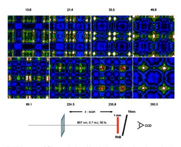
Fig. 79. Creation of space-controlled 2-D arrays of filaments by launching the beam through a wire mesh  $(11 \times 11 \text{ meshes}, \text{mesh } 497 \mu\text{m}, \text{wire}$  diameter 54  $\mu$ m). The characteristic diffraction patterns are shown for various distances. The shown image sections  $(1 \text{ mm} \times 1 \text{ mm})$  contain the center mesh and half of its neighbors (Schroeder et al., 2004).
