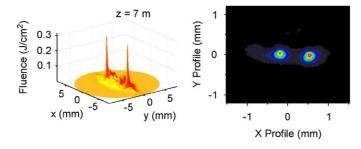
Fig. 77. Comparison of measured and simulated organized multiple filamentation patterns for an input beam with astigmatism (Méchain et al., 2004b).
