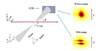
Fig. 57. Experimental diagram for time-resolved optical diffractometry, allowing the measurement of the filament size and the duration of the generated plasma. Note the fringes in the far field, when there is spatial and temporal overlap between the probe beam and the plasma column generated by the filament. From Tzortzakis et al. (2000a); Tzortzakis (2001).
