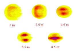
Fig. 56. Formation and fusion of twin filaments by an initially collimated laser beam (800 nm, 50 fs, 5 mJ). The transverse section of the beam is shown at various propagation distances. From Tzortzakis et al. (2001a).
