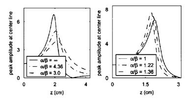
Fig. 44. Peak amplitude in the center of the pulse (r = 0, t = 0) for different amplitude ratio of the two input linearly polarized modes. According to Schjødt-Eriksen et al. (2001).
