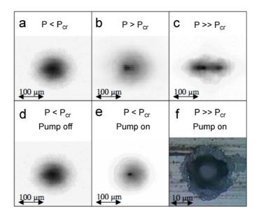
Fig. 91. Beam profile measured at the exit face of the crystal for several conditions. (a)  $P_{in} < P_{cr}$ , unpumped crystal; (b)  $E_{in} = 12 \,\mu$ J, unpumped crystal; (c)  $E_{in} = 47 \,\mu$ J, unpumped crystal; (d) same as (a); (e)  $E_{in} = 3.6 \,\mu$ J, pumped crystal; (f) image of the damage seen through a microscope (note the change of scale). In all cases, the pulse duration was 80 fs and the focus length of the lens was 8 cm. From Philip et al. (2005).
