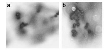
Fig. 101. Single-shot beam impacts on photosensitive papers after 75 m propagation in (a) dry air and (b) rain. The air pressure is 0.67 atm (altitude 3230 m). Filaments are clearly visible in both cases. The ring patterns on the profile in rain are due to the diffraction of the beam on the rain droplets.
