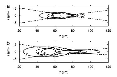
Fig. 50. Beam diameter in dashed curve (FWHM of the fluence at each propagation distance) and various levels of the fluence distribution (continuous contours for 1, 2, and  $3 \text{ J/cm}^2$  as a function of the propagation distance. Pulse: 800 nm, 160 fs. Focusing lens  $20 \times$  with NA = 0.5. (a) 0.45 µJ. (b) 1.1 µJ. From Couairon et al. (2005b).
