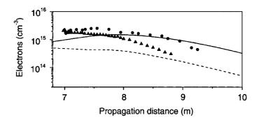
Fig. 74. Calculated and measured electron densities for a 2 mJ pulse with duration of 450 fs, (dashed line and triangles respectively), and for a 2 mJ pulse with duration of 5 ps, (solid line and circles respectively). From Tzortzakis et al. (2001b).
