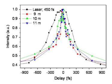
Fig. 60. Autocorrelation traces of an ultraviolet (248 nm) pulse (initial duration 450 fs) undergoing filamentation at various distances. From Tzortzakis et al. (2001b).
