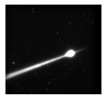
Fig. 2. Vertical propagation in the sky of the teramobile laser beam (peak power of 5 TW at 800 nm, see Section 5.1.1): backward scattering of the beam is recorded using the telescope with a 2 m aperture, located in Tautenburg, Germany. One distinguishes a zone of Mie scattering from a vapor cloud located at an altitude of 9 km.
