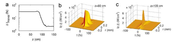
Fig. 29. (a) Pulse duration (FWHM) computed on the intensity integrated radially over 100  $\mu$ m during the filamentation of a 25 fs laser pulse in an argon pressure gradient. According to Couairon et al. (2005a). (b–c) Intensity distributions computed at the beginning (b) and at the end (c) of the pressure gradient.
