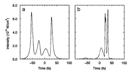
Fig. 28. On-axis pulse temporal profiles obtained by numerical simulations of filamentation in argon at 2.5 atm for a focused (f = 2 m), 60 fs, 1.2 mJ, 789 nm input pulse. (a) At the focal point and (b) 10 cm beyond the focus. According to Nurhuda et al. (2002a).
