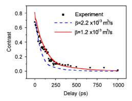
Fig. 64. Contrast of the probe wave front central fringe as a function of the delay between probe and self-guided pulse. The curves are obtained from the analytic formula (154). From Tzortzakis et al. (2000a).
