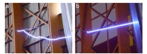
Fig. 94. Electric discharge between two electrodes separated by 4 m, with an applied difference of potential of 2 MV (a) and 1.7 MV (b). The rectilinear discharge is triggered by a filament connecting the two electrodes (Ackermann et al., 2005).
