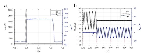
Fig. 105. (a) Voltage (dotted line) and current flowing (continuous line) between the two electrodes. The voltage is applied at t = 5.5 s during 1 s. The current discharge is triggered by the filaments.(b) Applied AC voltage (in kV units) and current flowing between the electrodes. The photodiode signal ( $U_{PhD}$ ) also gives the arrival time of the laser pulse on the electrode (at 1.05, 1.15 and 1.25 s).
