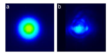
Fig. 11. Conical emission and laser pattern measured after 20 m of propagation in air from a 400 nm laser pulse. (a) Surrounding conical emission only, with the power spectrum close to that of the incident laser pulse removed by a colour filter. The external diameter of the blue ring is about 1 cm. (b) Strongly attenuated total laser beam at the same distance. From Prade et al. (2006a).
