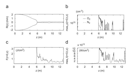
Fig. 23. Propagation of a collimated beam in air. The initial power of the pulse ( $\lambda = 800$  nm, duration = 50 fs) is about 25 P<sub>cr</sub>. (a) The diameter of the beam 2*R*, (b) the maximum density of free electrons, (c) the on axis fluence and (d) the peak intensity on axis are plotted as functions of the propagation distance. From Couairon et al. (2002).
