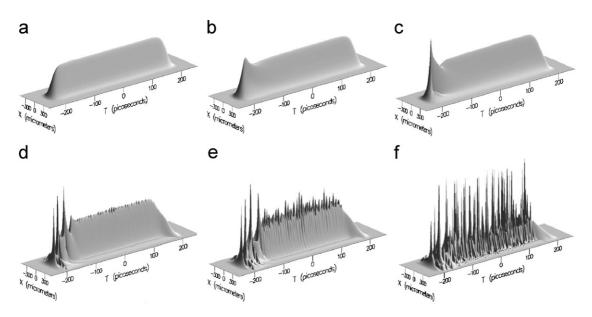
Fig. 26. Development of the modulational instability in the filamented ns pulse, leading to a train of shorter pulses (Niday et al., 2005).
