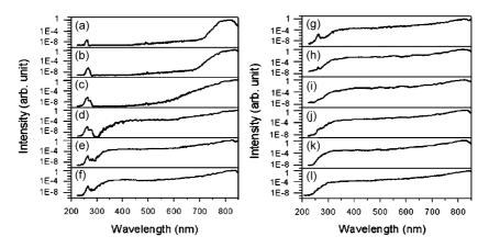
Fig. 63. Experimental spectrum of the third harmonic and fundamental continuum generated in atmospheric air at different pulse energies (a)  $250 \,\mu$ J, (b)  $500 \,\mu$ J, (c)  $750 \,\mu$ J, (d)  $1.0 \,\mu$ J, (e)  $1.25 \,\mu$ J, (f)  $1.5 \,\mu$ J, (g)  $1.75 \,\mu$ J, (h)  $2.0 \,\mu$ J, (i)  $3.0 \,\mu$ J, (j)  $4.0 \,\mu$ J, (k)  $5.0 \,\mu$ J and (l)  $10.0 \,\mu$ J using a lens of 380 cm focal length. From Théberge et al. (2005b, c).
