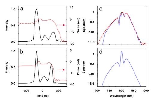
Fig. 47. (a) Axial intensity and phase measured with SHG-FROG. (b) Calculated axial intensity and phase. (c) Measured axial spectrum of field shown in (a). The curve is the square modulus of the Fourier transform of data in (a), while the points are measured with a spectrometer. (d) Calculated axial spectrum. From (Zozulya and Diddams, 1999).
