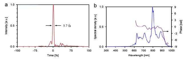
Fig. 61. Pulse self shortening by filamentation in argon gas cells. According to Hauri et al. (2004); Couairon et al. (2006a). (a) Temporal profile. (b) Spectral intensity (left axis) and phase (right axis).
