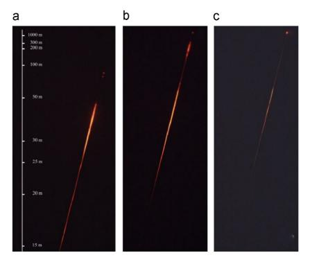
Fig. 96. Evolution of the white light continuum generation as a function of the propagation distance for different durations of the laser pulse: (a) 100 fs; (b) 1 ps; (c) 2 ps. From Méchain (2005).
