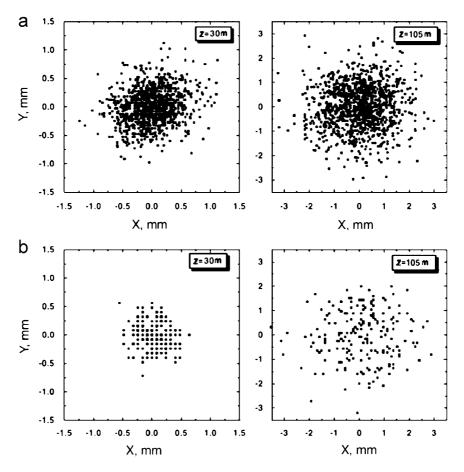
Fig. 38. Comparison between measured and calculated filament positions in the transverse diffraction plane at distances z = 30 and 105 m from the laser. (a) Experiments, 1100 shots. (b) Simulations 200 shots. From Chin et al. (2002b).
