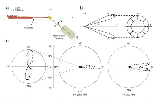
Fig. 70. (a) Experimental set-up for the measurement of THz emission. (b) Direction of the THz wave polarization in the emission cone. (c) Comparison between radial and forward THz emission from a filament. The polar diagram for the THz emission intensity as a function of the cone angle defined in (b) is shown for two different focal lengths f = 2 m (middle) and f = 75 cm (right). The radial emission (left) is magnified by a factor 100. From D'Amico et al. (2007b).
