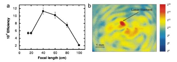
Fig. 67. (a) Conversion efficiency of the filamented pulse into its third harmonic, according to the propagation distance in the form of a filament. From Yang et al. (2003). (b) Typical transverse image of the UV light taken with a 12 bit CCD camera after 7 m of propagation in air (intensity scale is log2). From Alexeev et al. (2005).
