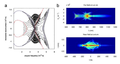
Fig. 55. (a) Contour plot of the logarithmic spectral intensity in  $(k, \omega)$  space for z = 1.7 cm after the first pulse splitting. From Kolesik et al. (2004). (b) Far-field (top) and near field (bottom) at a propagation distance of 4 cm for a 3.3 µJ infrared laser pulse undergoing filamentation in water. From Couairon et al. (2006c).
