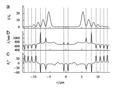
Fig. 53. (a) Transverse distribution of the beam intensity I(r, t=0) at 40 µm in front of the focus of a 45 fs, 3 µJ infrared laser pulsed beam focused in a water cell. (b) Wavelength of the supercontinuum sources  $\lambda(r, t=0) = 2\pi c/[\omega_0 + \Delta\omega(rt=0)]$ . (c) Divergence angle of their radiation  $\theta(r, t=0)$ . The pulse intensity is normalized to  $I_0 = 10^{12}$  W/cm<sup>2</sup>. From Liu et al. (2003a).
