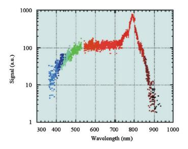
Fig. 8. Spectrum of a femtosecond laser beam ( $\lambda_0 = 800 \text{ nm}$ ;  $\tau_{FWHM} = 70 \text{ fs}$ ,  $P_{in} = 3 \text{ TW}$ ) after propagation over a distance of 10 m in air. The fast fall between 800 and 900 nm corresponds to the fall of the detectivity of the measuring apparatus (see Kasparian et al., 2000b).
