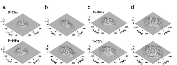
Fig. 78. Normalized three-dimensional views of filamentation patterns at z = 31 mm recorded with (a,c) a nearly circular incident beam (ellipticity e = 1.09) and (b,d) an elliptical incident beam (e = 2.2). The major axis of the ellipse lies along the *x*-axis of each plot.  $P_{cr} = 1.15$  MW in water, with 527 nm, 170 fs laser pulses. From Dubietis et al. (2004c).
