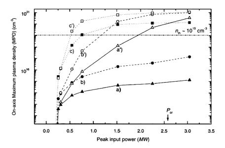
Fig. 48. Maximum plasma density at the physical focii in the bulk of a fused silica sample for: (a) 12 fs; (b) 36 fs; and (c) 120 fs pulses (filled symbols). The open symbols (a'), (b'), and (c') are the corresponding results when the focii are at the surface of the sample. From Junnarkar (2001).
