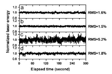
Fig. 12. Temporal evolution of energy per pulse normalized over the mean energy for (a) the infrared seed  $(1.1 \,\mu\text{m} < \lambda < 1.6 \,\mu\text{m})$ , (b) the near infrared pump pulse (807 nm), (c) the generated signal pulse for near infrared pump power (10 times below  $P_{cr}$  in air), and (d) the generated signal pulse for pump power of 2.5  $P_{cr}$ . The rms energy fluctuations are indicated on the right-hand side. From Théberge et al. (2006a).
