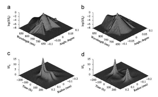
Fig. 31. Frequency angular spectrum (a, b) and spatio-temporal distribution (c, d) of the pulse at two propagation distances: (a, c)  $z = 0.43L_d$ ; (b, d)  $z = 0.6L_d$ . In the simulations the pulse duration was  $\tau_{\text{FWHM}} = 250$  fs, the input peak power was  $6.3P_{\text{cr}}$  and the input beam radius  $w_0 = 0.25$  mm. From Kandidov et al. (2003a).
