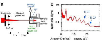
Fig. 58. (a) Principle for the measurement of the peak intensity in a filament. The odd harmonics generated in a cell filled with argon at low pressure are detected in a second cell filled with xenon. The energy of the free electrons in the xenon gas is measured by a detector of time of flight, which informs about the energy of VUV photons responsible for ionization. (b) The figure shows the odd harmonics ranging between the 11th and 23rd orders. From Lange (1998); Lange et al. (1998a).
