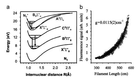
Fig. 73. (a) Schematic potential energy diagram for  $N_2$  and  $N_2^+$ . (b) Intensity of the fluorescence below 400 nm from nitrogen versus the filament length for an initially collimated laser beam. The solid line is the gain curve given by (157). From Luo et al. (2003, 2004).
