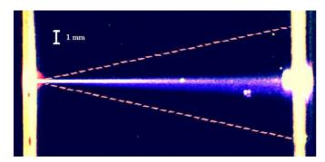
Fig. 81. Transverse photograph a 2 cm long filament generated in fused silica by focusing a 2 µJ, 800 nm, 160 fs laser pulse on the entrance face of the sample. From Tzortzakis et al. (2001d).
