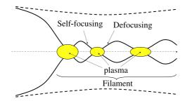
Fig. 6. Schematic representation of the focusing–defocusing cycles undergone by the intense core of the beam. The solid curves indicate the diameter of the intense core. The filamentation length is the distance covered by these cycles. The dashed line indicates the root mean square radius of the full beam.
