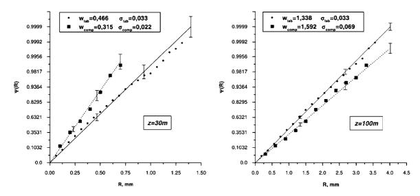
Fig. 39. Distribution function of the displacements of the filament center in the probability scale of the Rayleigh law. Solid curves: experiments. Dashed curves: simulations. The computed or measured averaged displacements are indicated for propagation distances of z = 30 and 105 m. From Chin et al. (2002b).
