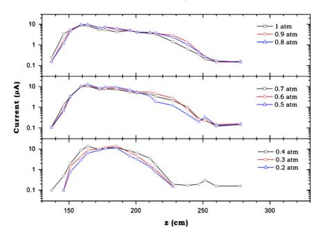
Fig. 75. Evolution of the conductivity of the filament along the optical axis with an energy equal to 3.7 mJ/pulse. *z* is the distance from the focusing lens. The presented signal corresponds to the current in the load resistance. The measurements have been performed for different pressures varying from 0.2 to 1 atm. From Méchain et al. (2006) and Méchain (2005).
