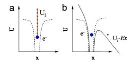
Fig. 5. Schematic diagram of: (a) multiphoton and (b) tunnel ionization.
