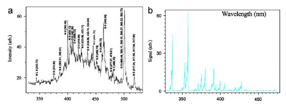
Fig. 71. (a) Nitrogen spectrum for a hot plasma with continuum and atomic lines. (b) Fluorescence spectrum of air interacting with Ti:sapphire laser pulses. According to Talebpour et al. (1999a).
