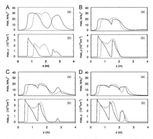
Fig. 16. (a) On-axis peak intensity and (b) peak electron density vs. propagation distance for  $P_{in}/P_{cr} = 4$  (A), 6 (B), 6.5 (C) and 7 (D). The continuous curves correspond to the inclusion of the Raman–Kerr contribution in the model while for the dashed curves, it is omitted. From Mlejnek et al. (1999c).
