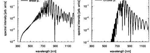
Fig. 46. Spectral broadening of two femtosecond pulses with different initial polarizations. The linearly polarized pulse (a) produces significantly more supercontinuum light than an equally intense circularly polarized pulse (b). From Kolesik et al. (2001).
