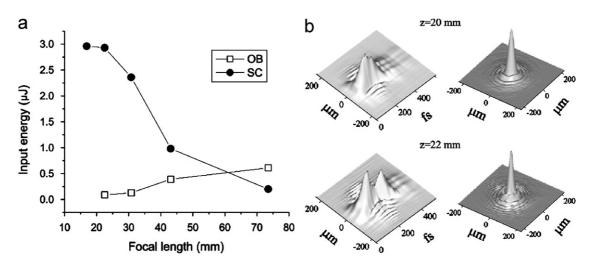
Fig. 85. (a) Threshold energies for supercontinuum generation (SC, filled circles) and optical breakdown (OB, open squares). From Liu et al. (2003b). (b) Measured space–time intensity profiles (left) and (time-integrated) normalized fluence profiles (right) for different propagation distances of a 150 fs, 527 nm laser pulse undergoing filamentation. From Matijošius et al. (2004b).
