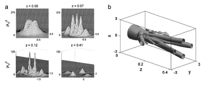
Fig. 37. Numerical simulation of vectorial and nonparaxial multiple filamentation for an input beam having  $P_{in} = 20P_{cr}$  and a nonparaxiality parameter of  $\epsilon \equiv 1/kw_0 = 0.08$ . (a) The normalized intensity is shown at different propagation distances, normalized to the Rayleigh length. (b) The iso-surface of the normalized intensity shows the multiple filaments. From Fibich and Ilan (2001b).
