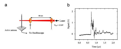
Fig. 100. (a) Experimental set up to measure the radiation at long wavelength from a plasma column in air (see text for details). (b) Signal detected by an antenna active between 10 kHz and 30 MHz. The signal corresponds to the average of 8 successive recordings. From Méchain et al. (2005c).
