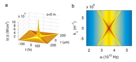
Fig. 17. (a) Near field (r, t) profile of an X-wave. (b) Far-field  $(k_{\perp}, \omega)$  of the X-wave shown in (a).
