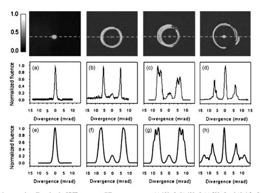
Fig. 68. TH pictures and profiles taken by ICCD camera at different pump energy (a)  $100 \,\mu$ J, (b)  $400 \,\mu$ J, (c)  $500 \,\mu$ J and (d)  $1.3 \,m$ J using  $100 \,cm$  focal length lens. Simulated spatial profile of the TH at different pump energy (e)  $85 \,\mu$ J, (f)  $340 \,\mu$ J, (g)  $510 \,\mu$ J and (h)  $1.278 \,m$ J. From Théberge et al. (2005a).
