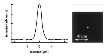
Fig. 104. Waveguide output profile at 633 nm. A near-field image is shown on the right-hand side. From Yamada et al. (2001).
