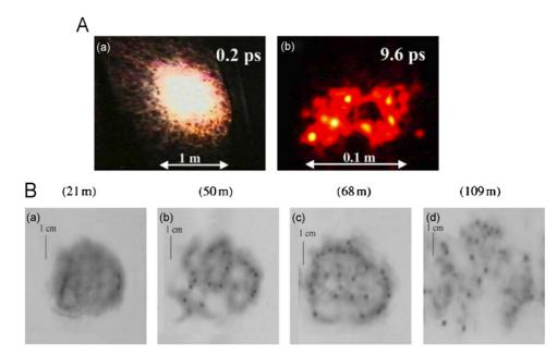
Fig. 97. (A) Comparison between two beam cross-sections at 1000 m. (a) minimum negative chirp: 0.2 ps, (b) maximum negative chirp: 9.6 ps. (B) Measured beam profile at various distances with a initial pulse duration stretched to 1.2 ps. From Méchain et al. (2005a).
