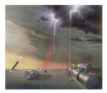
Fig. 102. Artistic view of possible scheme to trigger and guide lightning with a laser. (a) powerful long laser pulse induce a plasma ball at a finite propagation distance. (b) Dashed lightning rod made up of a collection of plasma balls generated by successive long laser pulses. (c) Potential straight lightning rod from earth to cloud generated by a filamenting ultrashort laser pulse. From Diels et al. (1997).
