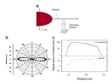
Fig. 69. (a) General diagram for the detection of the sub-THz radiation from a plasma channel generated by a filament. (b) The radiation diagram shows two lobes with an intensity maximum. The lobes are perpendicular to the axis of the filament (Tzortzakis et al., 2002). (c) Comparison of filamentation lengths measured by conductivity and by sub-THz detection.
