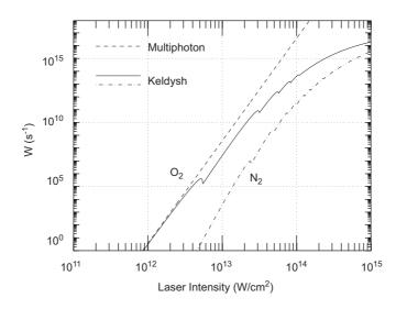
Fig. 20. Ionization rates for oxygen (continuous curve) and nitrogen (dash-dotted curve) vs. laser intensity at 800 nm. The dashed line shows the multiphoton ionization rate of oxygen.
