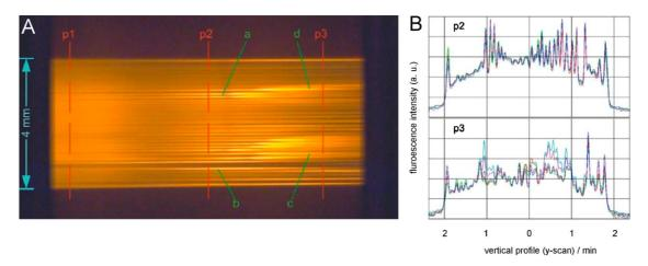
Fig. 89. (A) Development of a one-dimensional filament array in methanol behind a slit from a 23  $\mu$ J (200  $P_{cr}$ ), 46 fs, 810 nm laser pulse. The yellow color is the two-photon fluorescence from Rhodamine B which was added to monitor the local intensity of the propagation of the initially collimated, transform limited femtosecond Ti–sapphire laser beam. (B) Five profile scans in the same day were taken at positions p2 and p3. From Schroeder and Chin (2004).
