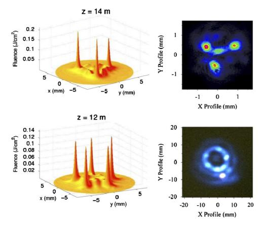
Fig. 76. Comparison of measured and simulated organized multiple filamentation patterns. A trefoil mask was used for the first line while a five-foil mask was used for the second (Méchain et al., 2004b).
