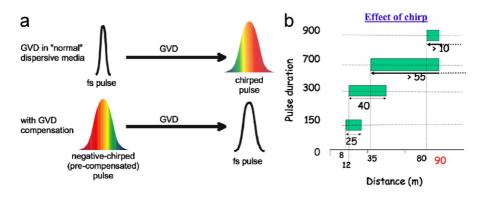
Fig. 98. (a) Principle of the GVD compensation. (b) Filamentation distance as a function of the duration of the laser pulse. The lengthening of the laser pulse is obtained by adding a negative chirp to the pulse. The optical Kerr effects dominates dispersion at high powers. From Méchain et al. (2005a).
