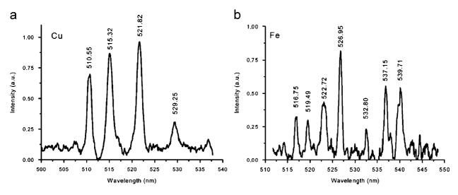
Fig. 103. LIBS spectra of copper (a) and steel (b), measured at 90 m distance (Stelmaszczyk et al., 2004).
