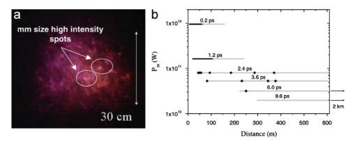
Fig. 95. (a) Beam cross section intercepted by a white screen at a propagation distance of 2350 m. The initial negative chirp corresponded to a duration of 9.6 ps. (b) Filamentation length as a function of the chirp of the input laser pulse. The duration of the non-chirped pulse is 100 fs. Black points and lines refer to locations where air ionization could be detected, gray lines to distances where bright light channels were observed. According to Méchain et al. (2005a, 2004a).
