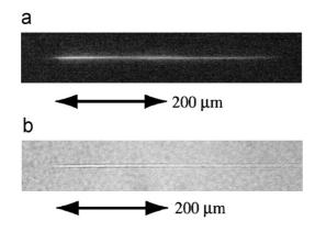
Fig. 84. Relationship between a filament and the region of refractive-index change: optical images of (a) the filament and (b) the region of refractive-index change. From Yamada et al. (2001).
