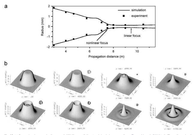
Fig. 27. (a) Comparison between the diameter of a UV filament (248 nm) and simulations, according to Tzortzakis et al. (2001b). (b) Three-dimensional fluence simulated profiles for different distances. Insets: experimental burning spots of the laser on photographic paper at the same distances. The sizes of the burning spots are not to scale. From Tzortzakis et al. (2000b, 2001b).
