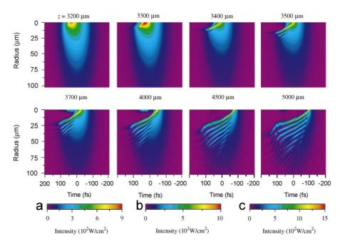
Fig. 51. Spatiotemporal intensity distribution of an initially Gaussian pulse with an energy of 135  $\mu$ J propagating in silica at eight different propagation distances *z* indicated above each image. The colormap (a) of intensity applies for *z* = 3200 m, (b) for *z* = 3300 m, and (c) for the other values of *z*. From Ishikawa et al. (2002).
