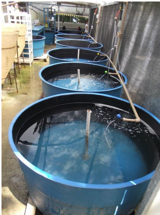
Appendix 4.3: Structures of the flow-through system consisting of three cylindrical rearing tanks of paralarvae (a control tank and two replicas) each 1 000 L, kept at the University of São Paulo's Center for Marine Biology (CEBimar) near the São Sebastião Channel.
