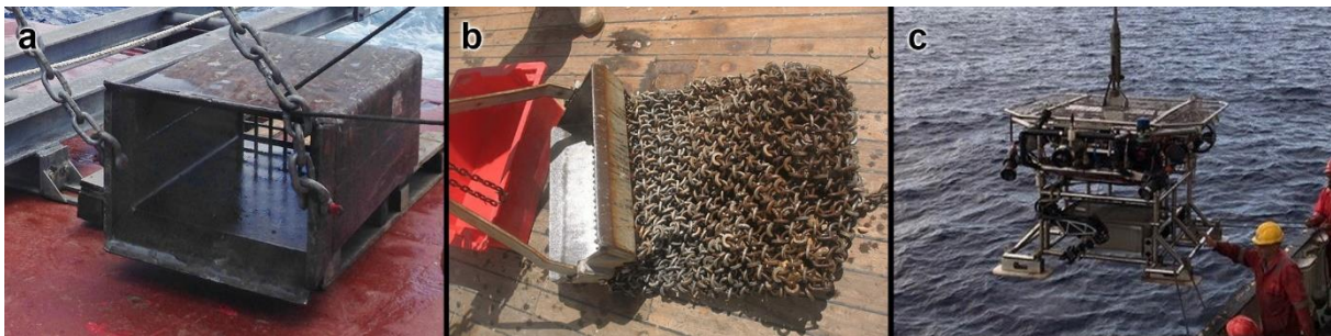
Figure 3.1. Sampling devices used in the N/Oc. Alpha Crucis (RGR1) (a) and RSS Discovery (DY94) (b and c) cruises. (a) Squared rock dredge with a meshed bottom. (b) Rectangular rock dredge with a collection bag of interlaced metal rings. Source: Rees et al. (2009). (c) RUV HyBIS being deployed in the water.
