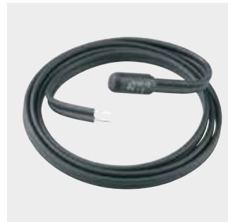
Temperature sensor 700802201 ● Resolution 1 °C, B-value 3435 K ± 1%, 10 kΩ at 25 °C, black (similar RAL 9005), 600 mm, 6 g
