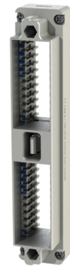
Receiver, i2 MX, 2 SIM Module Inserts, 22 Position, EMI-Shielded Part # 310 130 113
