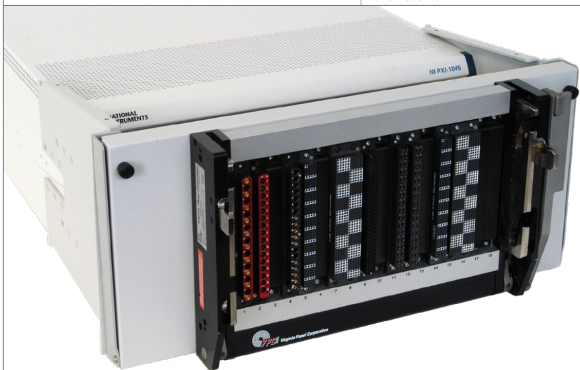
G18 Mounted to Vertical Hinged Mounting Frame
