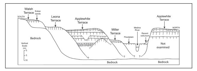
Figure 3.1. Schematic cross-section of the Medina River valley showing the terraces, underlying deposits, and soils.
