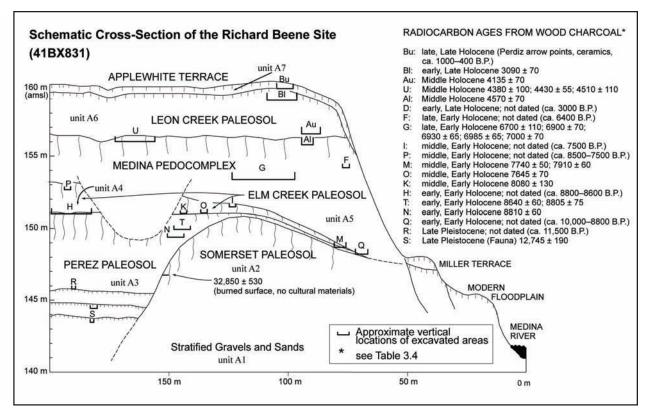
Figure 9.3. Schematic profile, showing paleosol stratigraphic units (Chapter 3), approximate statigraphic positions and radiocarbon ages of block excavation areas and cultural-period designations.
