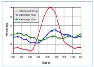
Fig. 13. Heat storage underneath of the roof collector using water-filled black tubes [24].
