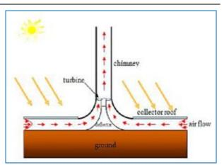
Fig. 1. Schematic diagram of solar chimney [1].
