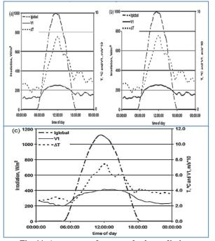
Fig. 11. An average of measured solar radiation, temperature and velocity. (a) For selected 5 clear days of October (with turbine installed), (b) for selected 6 clear days between 19 and 30 October (with turbine removed), (c) for 6 days between 14 and 21 November (with turbine and diffuser removed) [17].
