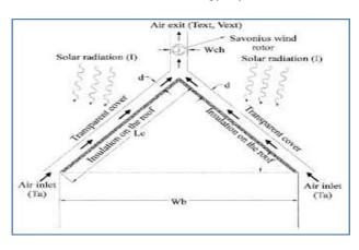
Fig. 23. Schematic of roof- top solar chimney [34].
