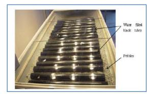
Fig. 19. The solar collector layout [31].
