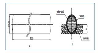
Fig. 20. Profile chart of thermal storage in the solar collector [31], (a) The dimension of water tube for thermal storage material, (b) Cross- section of water in radial.
