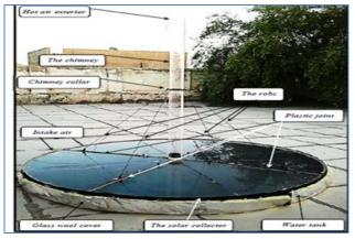
Fig. 25. Photograph of the experimental scale model of the solar chimney power plant by Hiader [36].
