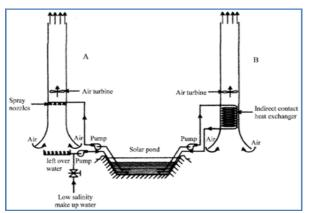
Fig. 16. Concepts for combining a chimney with a solar pond to generate power [28].
