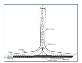
Fig. 17. Structure diagram of solar chimney – sea desalination integrated system [30].
