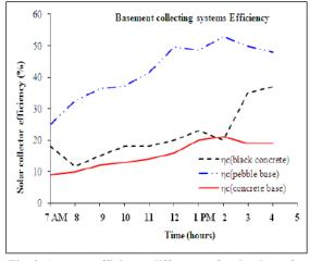
Fig. 8. Average efficiency differences for day hour for basement system [12].
