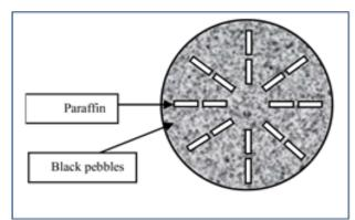
Fig. 33 b. Second model with rectangular containers.
