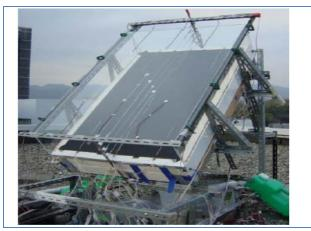
Fig. 29. Photograph of the prototype solar chimney with PCM modules for natural ventilation [44].
