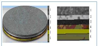
Fig. 5. Description of the special ground layer (1. Asphalt, 2.Glass, 3. Thick sand 4. Gravel 5. Aluminum foil with glass wool 6. Ground floor). [11].
