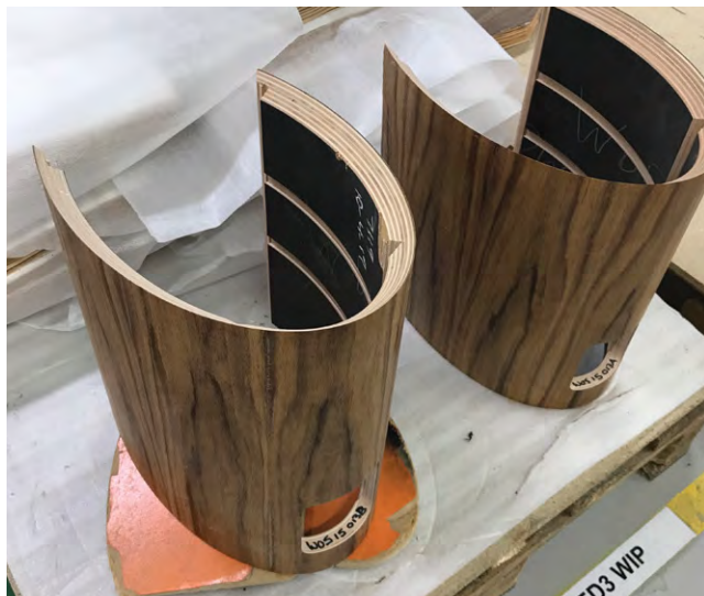
A partially finished cabinet shows the wood layers.
