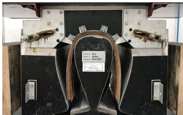
In the second step, the layers of wood are put into a press and held there until the adhesive cures and the wood/glue assembly has been bent into a rounded cabinet shape.
