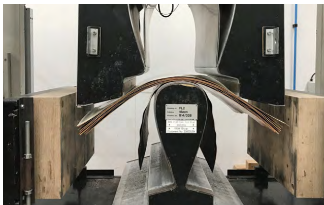
A speaker cabinet being made using B&W's Reverse Wrap technology. In the first step, thin layers of wood are stacked together with an industrial adhesive between the layers.
