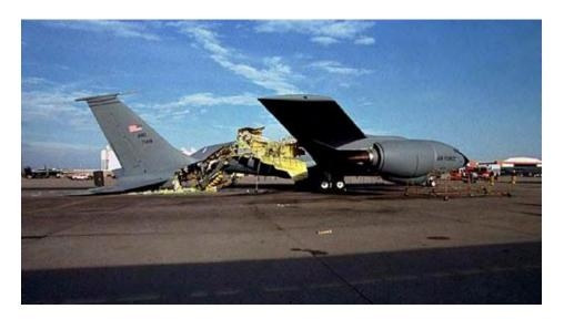
7 April - A KC-135R Stratotanker, 57-1418, of the 151st Air Refueling Squadron, Tennessee Air National Guard, is written off while undergoing maintenance at the Oklahoma ALC, Tinker AFB, Oklahoma, when the cabin is over-pressurized during a test and ruptures, tearing a 35 foot (10.6 m) hole in the aft fuselage, allowing tail section to drop to the ground.
