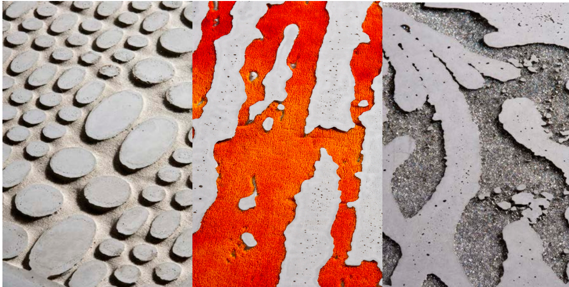
Figure 1: From left to right: Linen and Concrete, Velvet and Concrete, Crystal Bead and Concrete (Images are Tactility Factory Ltd. Copyright).
