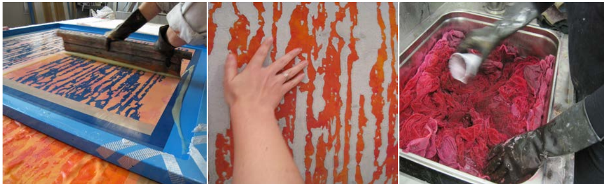
Figure 1: From left to right: Devore Printing Velvet, Finished Velvet Concrete Surface, Hand Dyeing (Images are Tactility Factory Ltd. Copyright).
