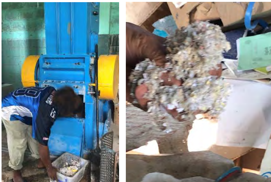
Figure 11: Paper shredder at the National Redemption Center (left) and shredded paper (right). (Source: APWC, 2019)
