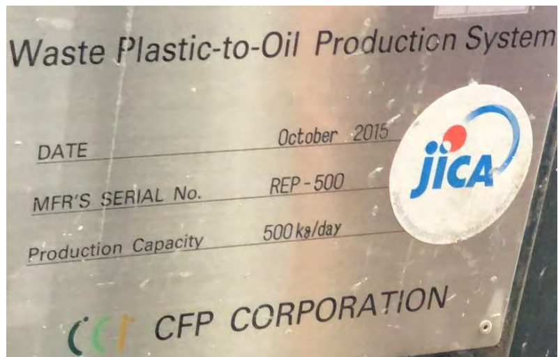
Figure 13: Pyrolysis machine's plaque at the National Redemption Center, Palau showing details. (Source: APWC, 2019)
